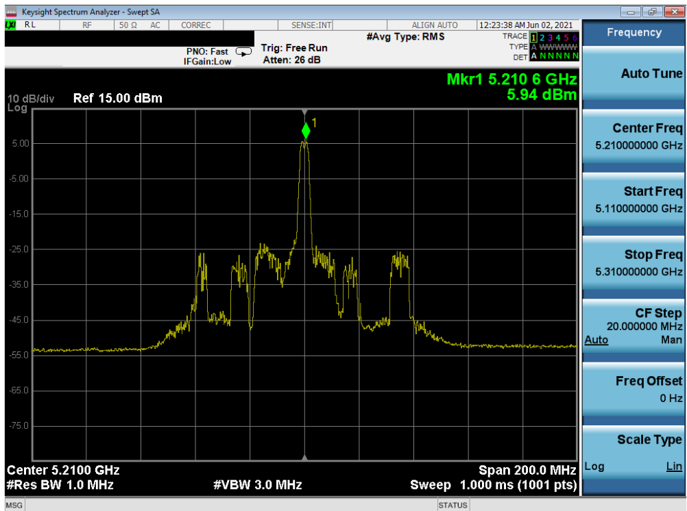
Plot 7-438. Power Spectral Density Plot MIMO ANT1 (80MHz BW 802.11ax – 26 Tones (UNII Band 1) – Ch. 42)
