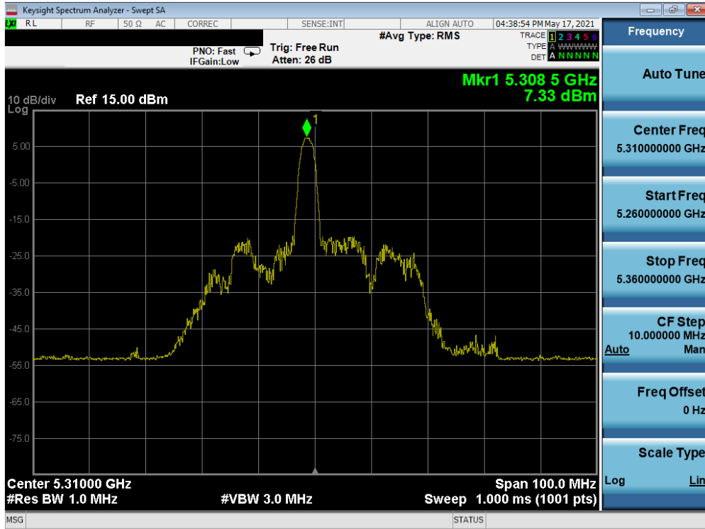
Plot 7-281. Power Spectral Density Plot SISO ANT1 (40MHz BW 802.11ax – 26 Tones (UNII Band 2A) – Ch. 62)
