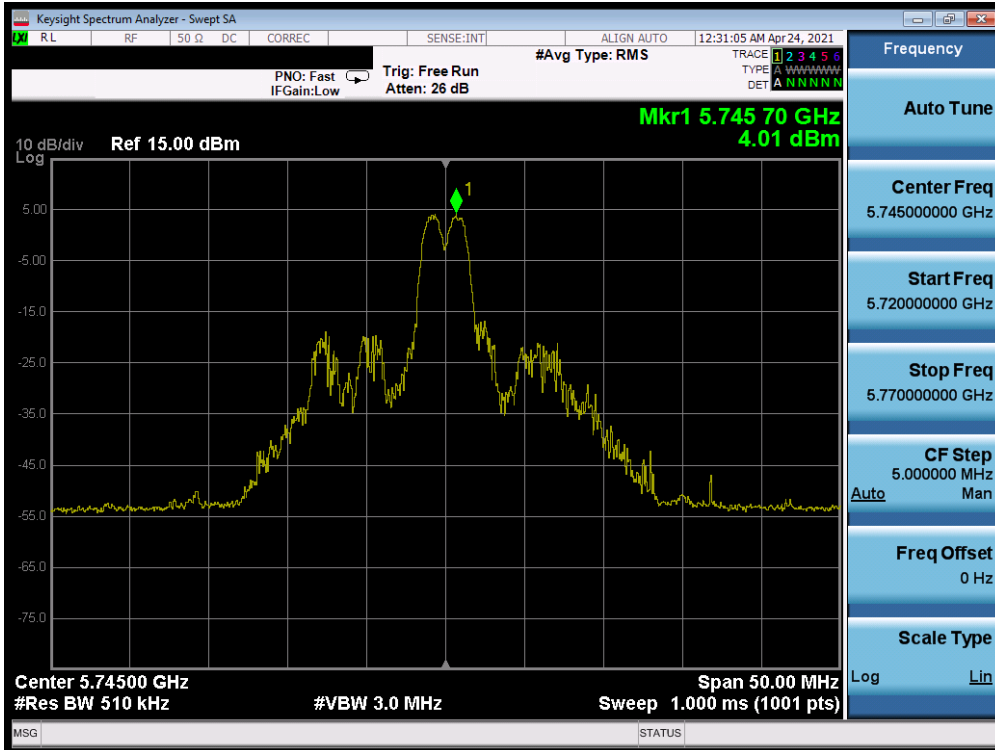
Plot 7-346. Power Spectral Density Plot MIMO ANT1 (20MHz BW 802.11ax – 26 Tones (UNII Band 3) – Ch. 149)
