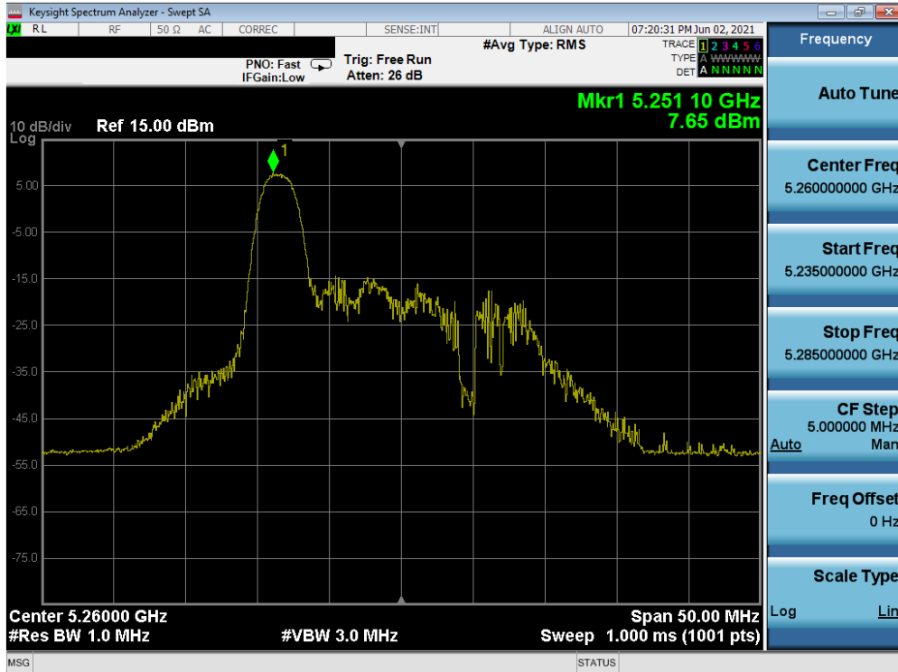
Plot 7-358. Power Spectral Density Plot MIMO ANT2 (20MHz BW 802.11ax – 26 Tones (UNII Band 2A) – Ch. 52)
