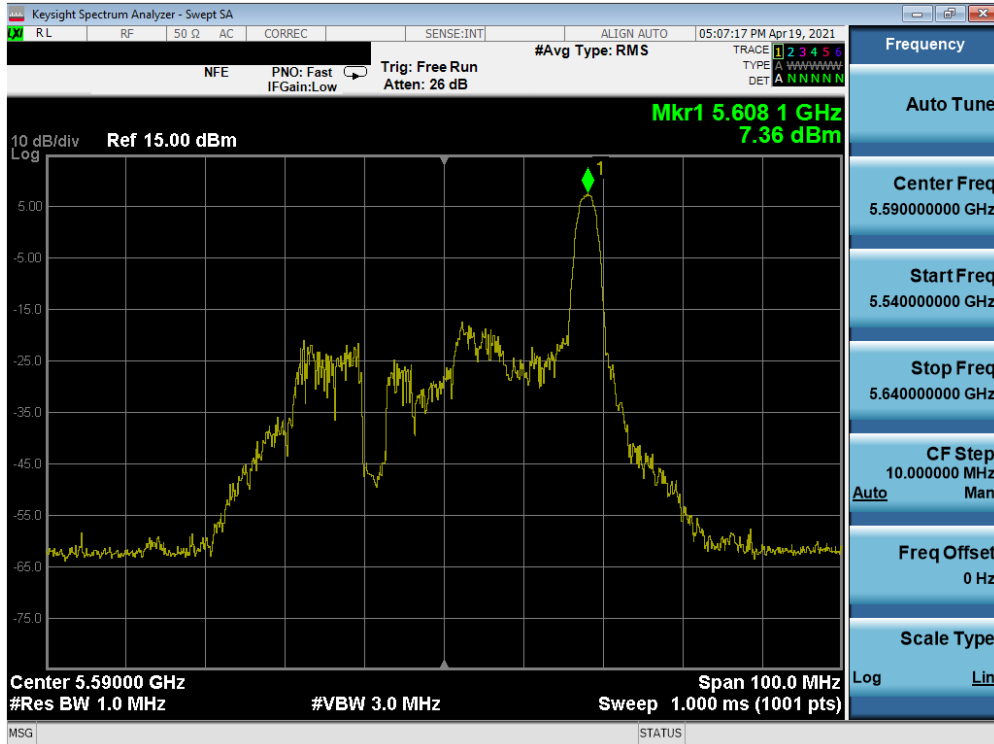
Plot 7-233. Power Spectral Density Plot SISO ANT1 (40MHz BW 802.11ax – 26 Tones (UNII Band 2C) – Ch. 118)
