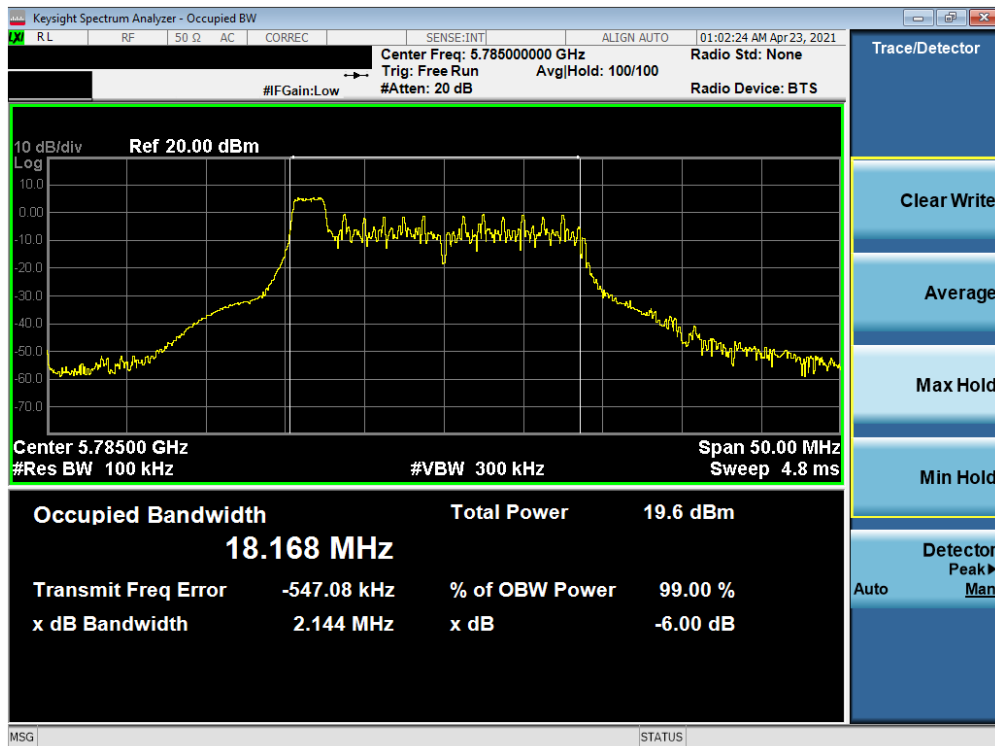
Plot 7-194. 6dB Bandwidth Plot SISO ANT1 (20MHz BW 802.11ax – 26 Tones (UNII Band 3) – Ch. 157)
