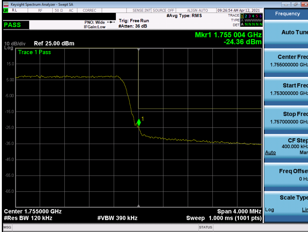
Plot 7-119. Upper Band Edge Plot (LTE Band 4 - 5MHz QPSK – Full RB)
