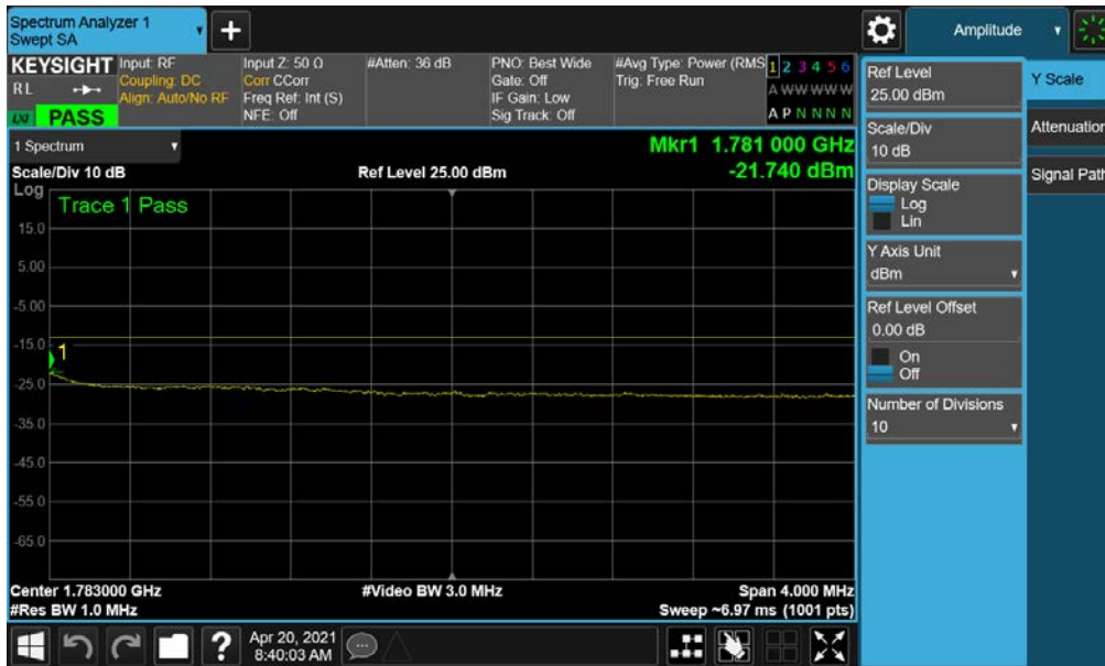
Plot 7-142. Upper Extended Band Edge Plot (NR Band n66 – 15.0MHz - Full RB)
