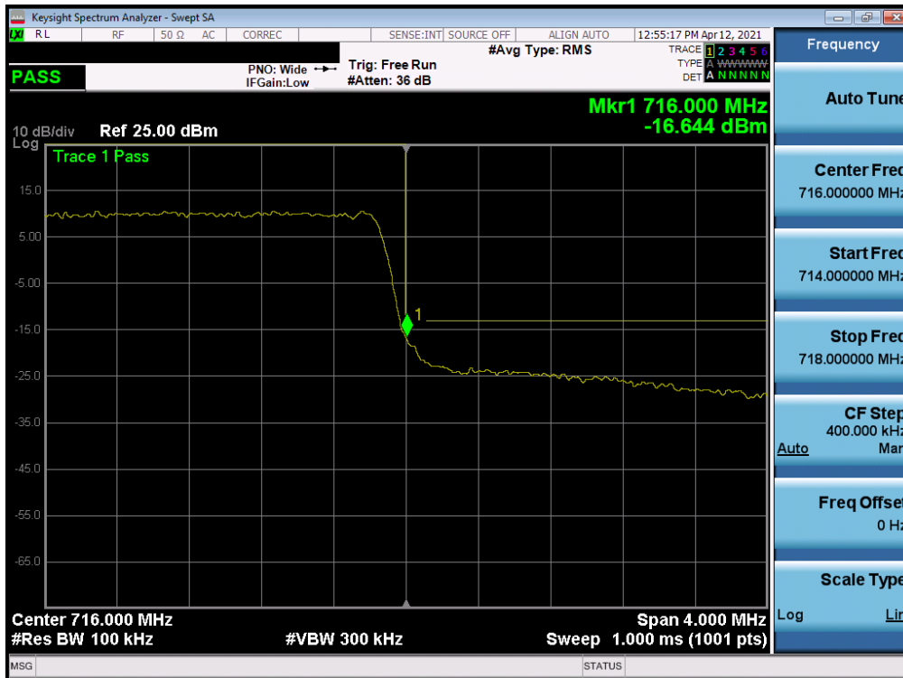
Plot 7-84. Upper Band Edge Plot (LTE Band 12 - 3MHz QPSK – Full RB)
