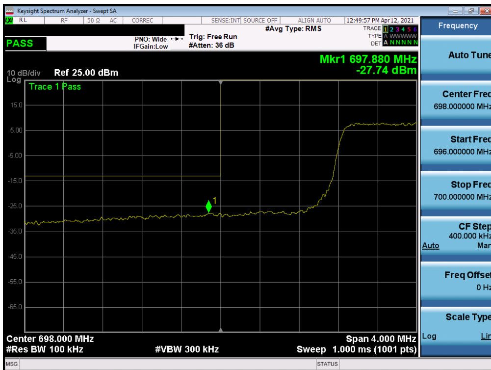
Plot 7-80. Lower Band Edge Plot (LTE Band 12 - 5MHz QPSK – Full RB)
