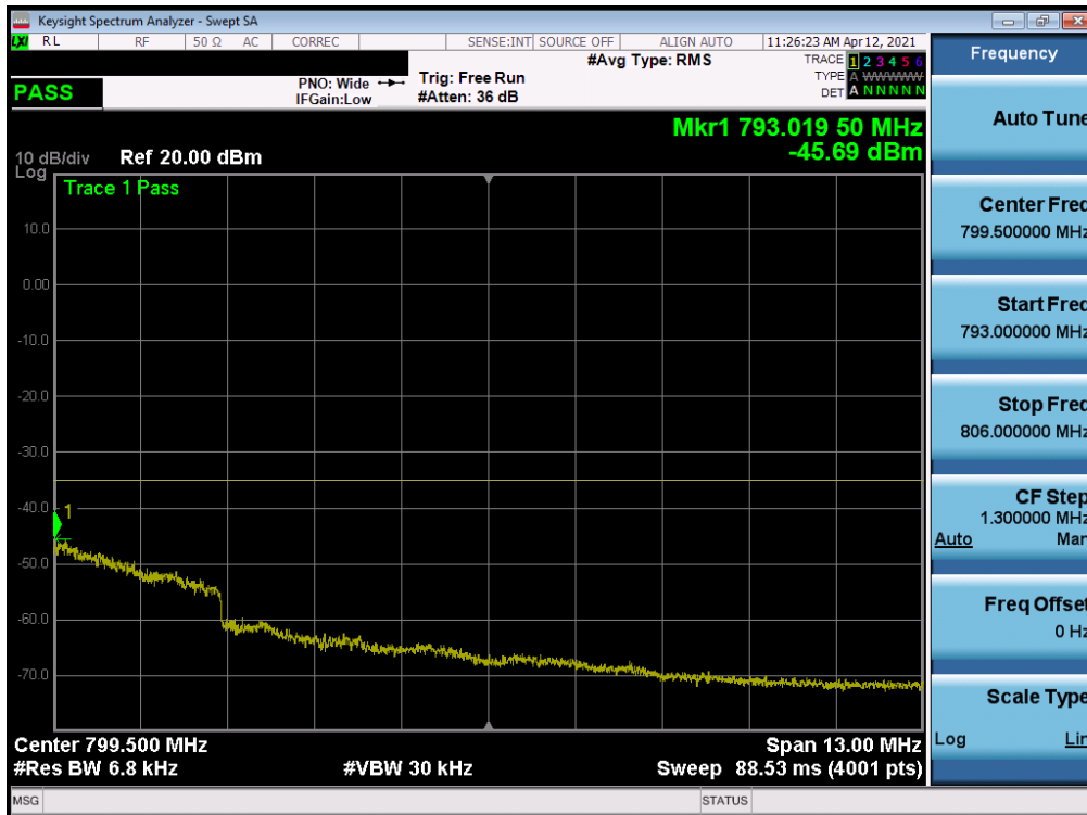
Plot 7-90. Upper Emission Mask Plot (LTE Band 13 - 10MHz QPSK – Full RB)
