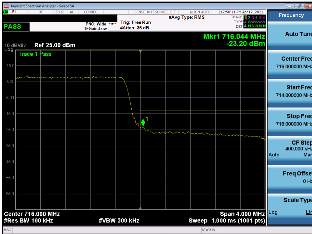
Plot 7-82. Upper Band Edge Plot (LTE Band 12/17 - 5MHz QPSK – Full RB)
