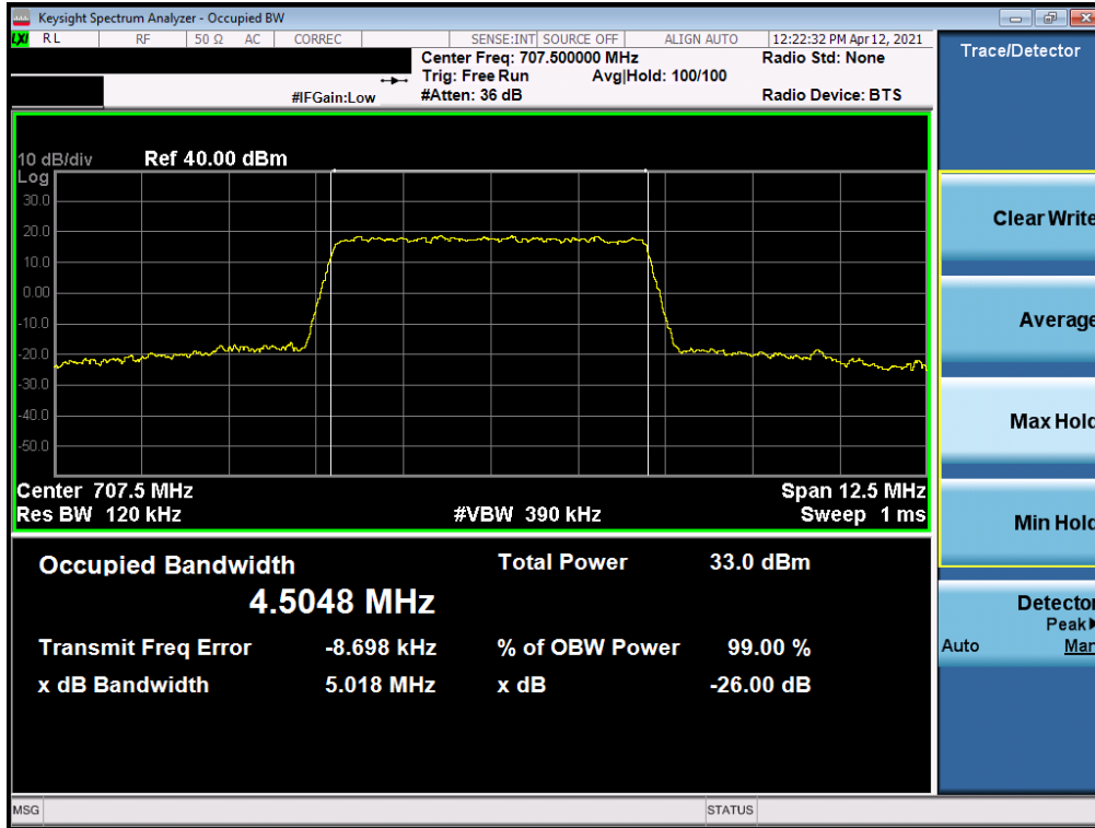
Plot 7-3. Occupied Bandwidth Plot (LTE Band 12/17 - 5MHz QPSK - Full RB)
