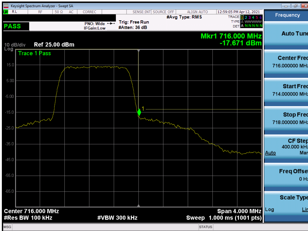
Plot 7-86. Upper Band Edge Plot (LTE Band 12 – 1.4MHz QPSK – Full RB)
