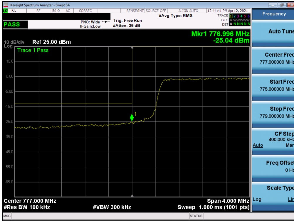
Plot 7-87. Lower Band Edge Plot (LTE Band 13 - 10MHz QPSK – Full RB)
