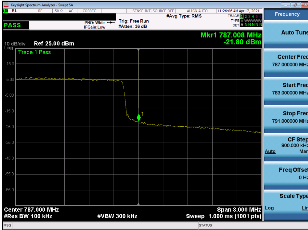
Plot 7-89. Upper Band Edge Plot (LTE Band 13 - 10MHz QPSK – Full RB)
