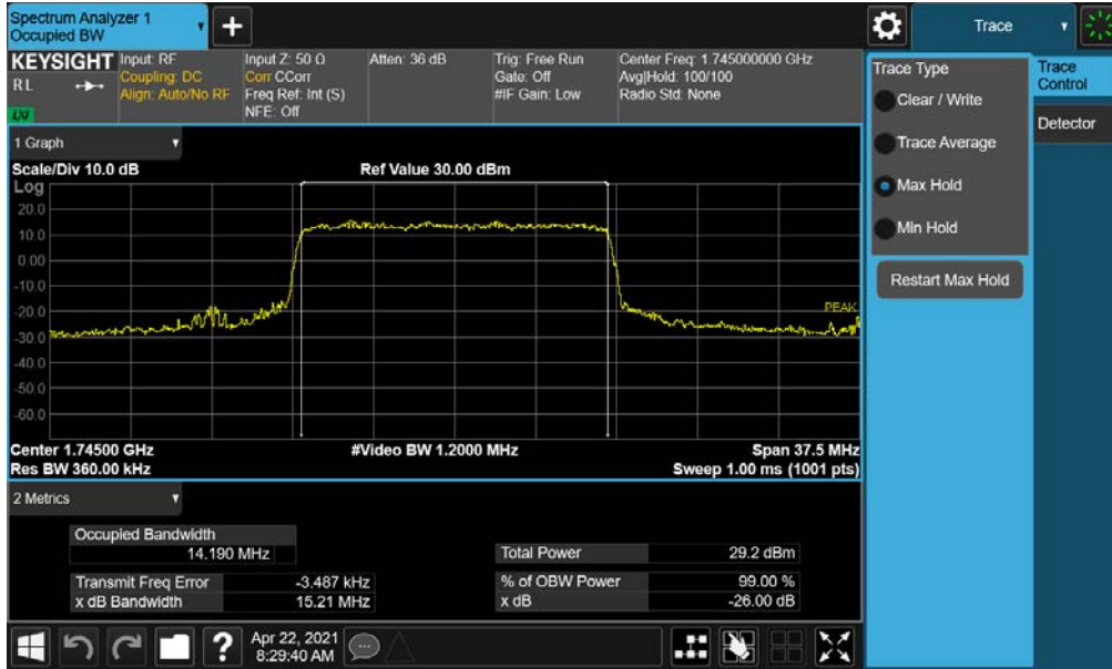
Plot 7-30. Occupied Bandwidth Plot (NR Band n66 - 15.0MHz CP-OFDM QPSK - Full RB)
