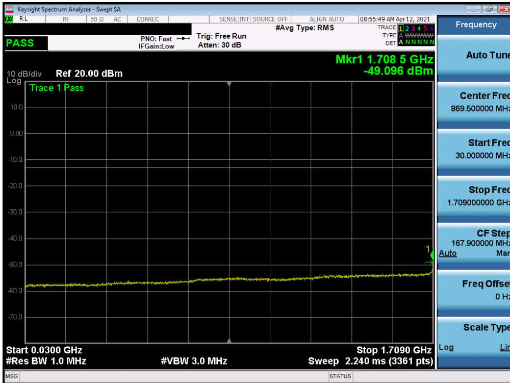
Plot 7-59. Conducted Spurious Plot (LTE Band 66/4 - 20MHz QPSK - RB Size 1, RB Offset 0 - Low Channel)
