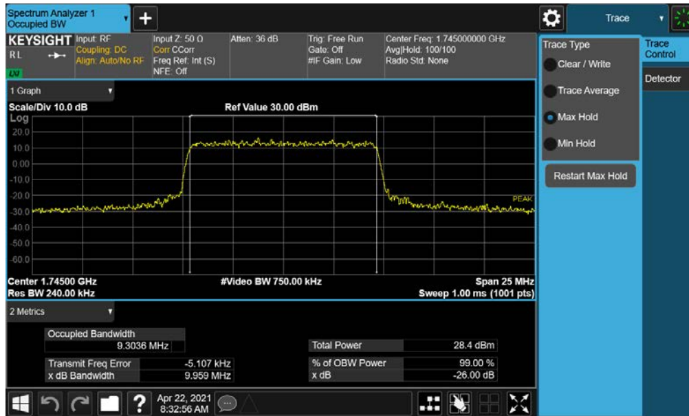
Plot 7-34. Occupied Bandwidth Plot (NR Band n66 - 10.0MHz CP-OFDM 16QAM - Full RB)
