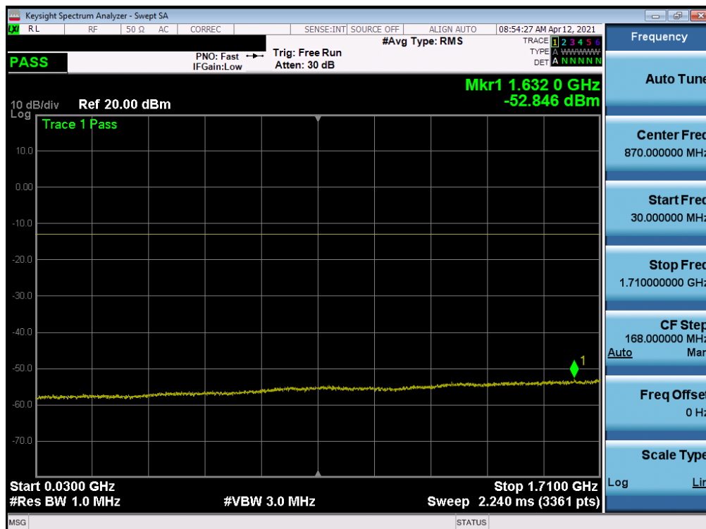
Plot 7-62. Conducted Spurious Plot (LTE Band 66/4 - 20MHz QPSK - RB Size 1, RB Offset 0 - Mid Channel)
