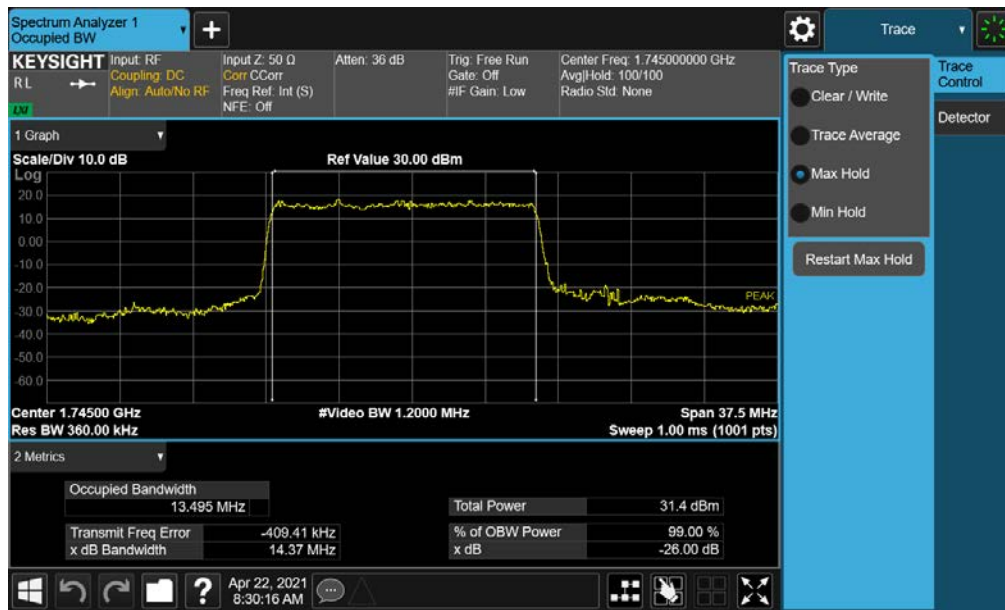
Plot 7-29. Occupied Bandwidth Plot (NR Band n66 - 15.0MHz \pi/2 BPSK - Full RB)
