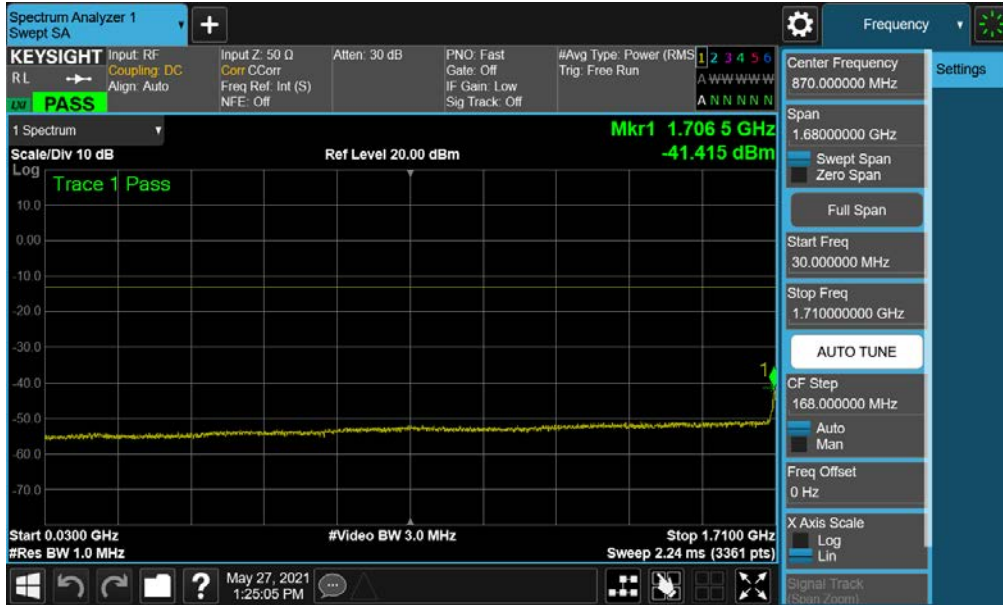
Plot 7-68. Conducted Spurious Plot (NR Band n66 - 20.0MHz - RB Size 1, RB Offset 0 - Low Channel)
