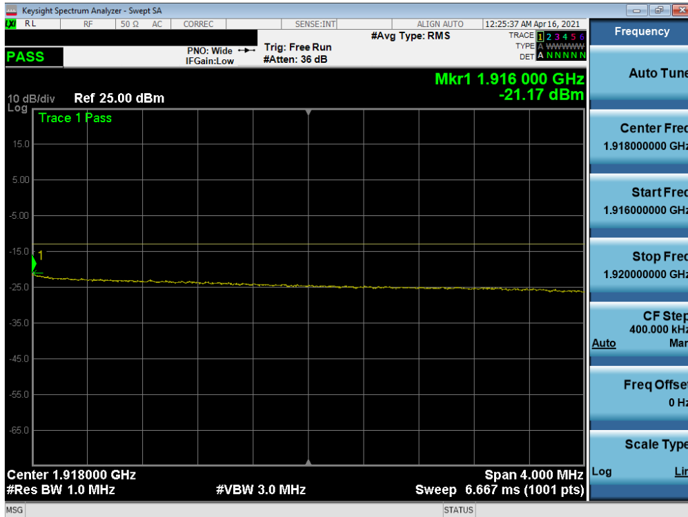
Plot 7-60. Extended Upper Band Edge Plot (LTE Band 25 - 10MHz QPSK – Full RB)
