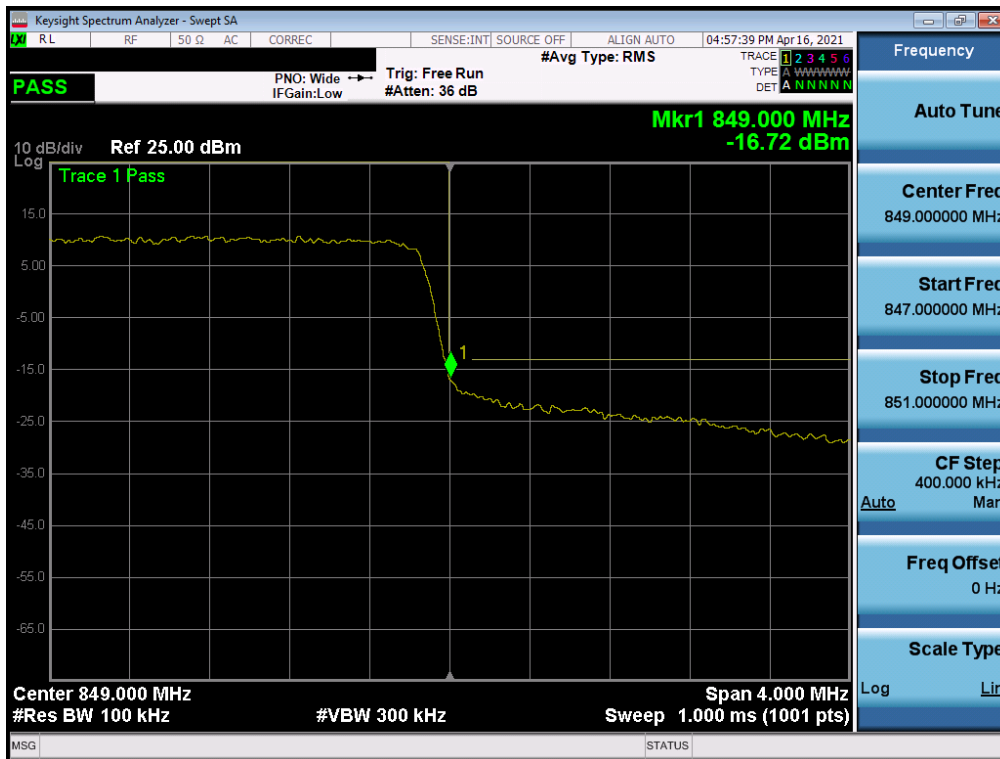
Plot 7-63. Upper Band Edge Plot (LTE Band 26/5 - 3MHz QPSK – Full RB)
