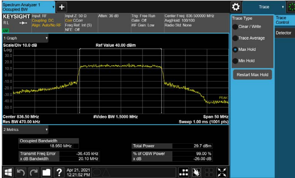
Plot 7-13. Occupied Bandwidth Plot (NR Band n5 - 20MHz 16-QAM - Full RB)
