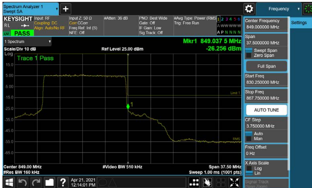
Plot 7-69. Upper Band Edge Plot (NR Band n5 – 15.0MHz - Full RB)
