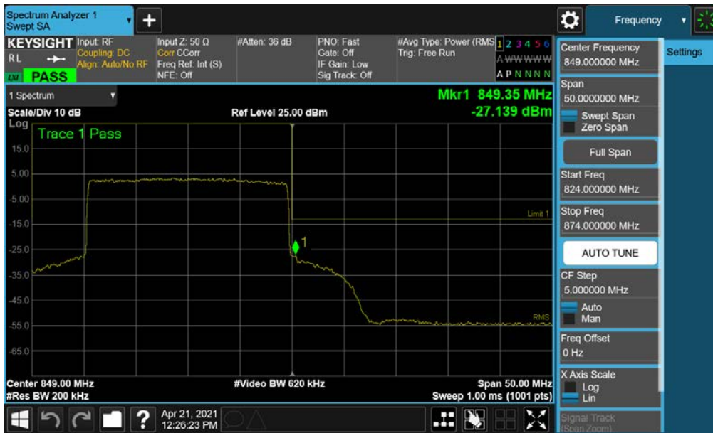
Plot 7-67. Upper Band Edge Plot (NR Band n5 – 20.0MHz - Full RB)
