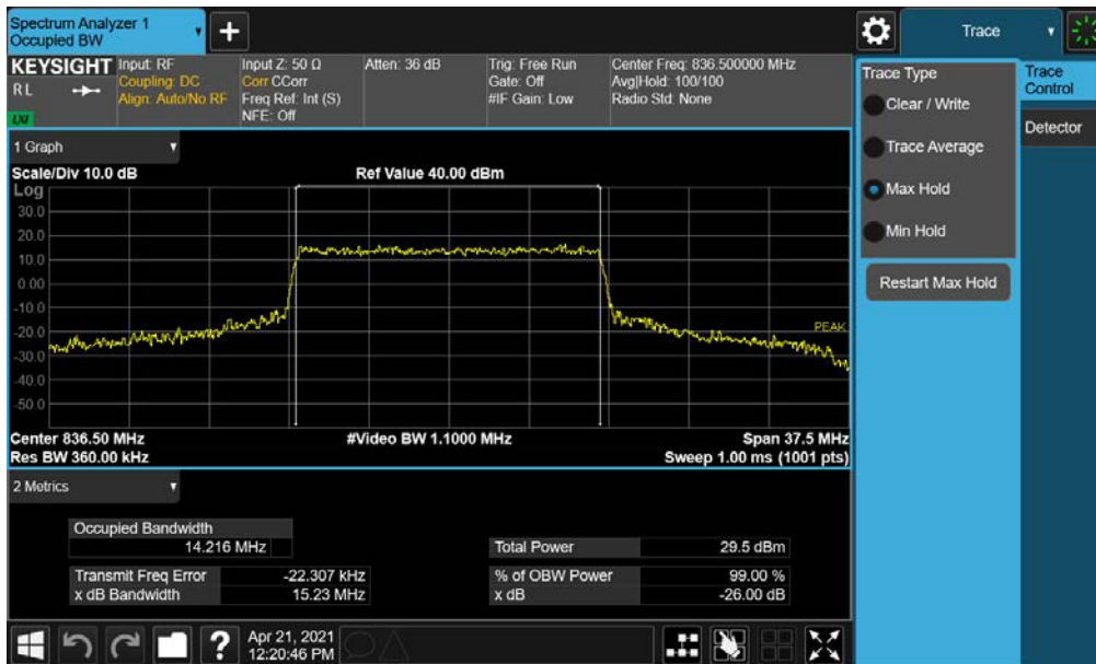
Plot 7-16. Occupied Bandwidth Plot (NR Band n5 - 15MHz 16-QAM - Full RB)
