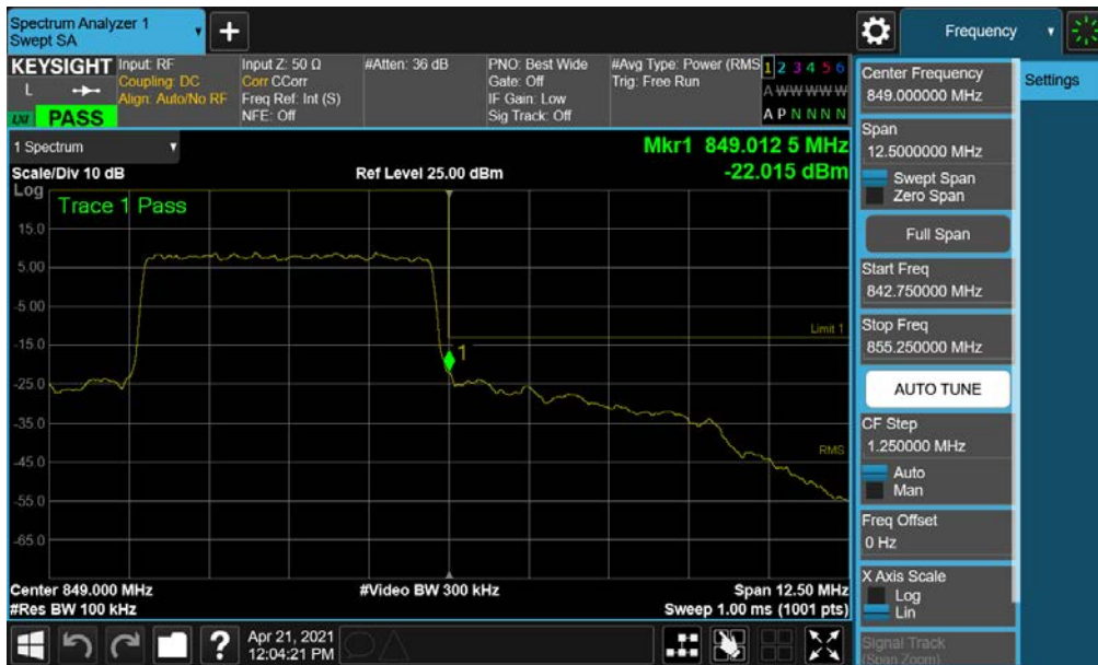
Plot 7-73. Upper Band Edge Plot (NR Band n5 – 5.0MHz - Full RB)
