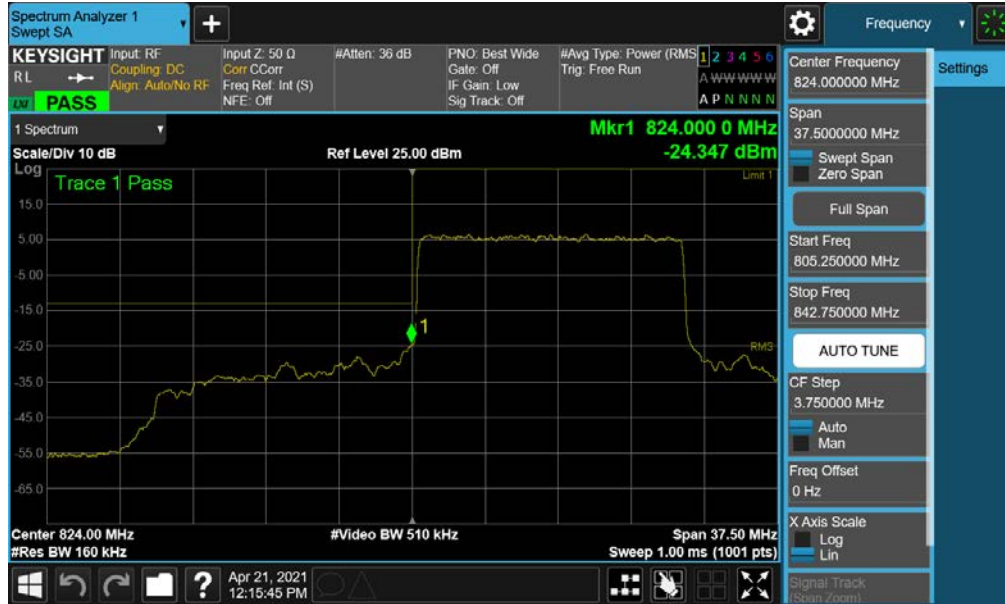
Plot 7-68. Lower Band Edge Plot (NR Band n5 – 15.0MHz - Full RB)
