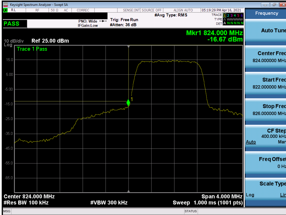
Plot 7-64. Lower Band Edge Plot (LTE Band 26/5 – 1.4MHz QPSK – Full RB)
