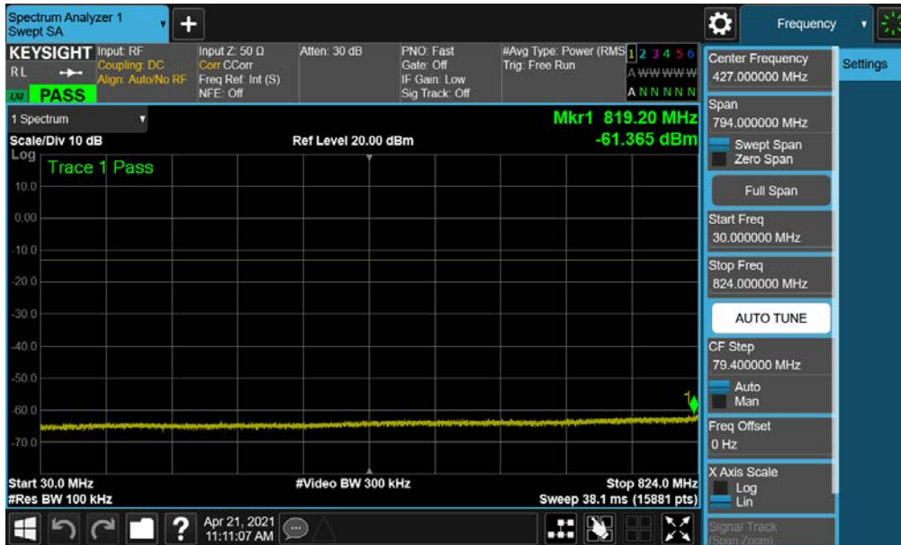
Plot 7-35. Conducted Spurious Plot (NR Band n5 - 20.0MHz - 1 RB)
