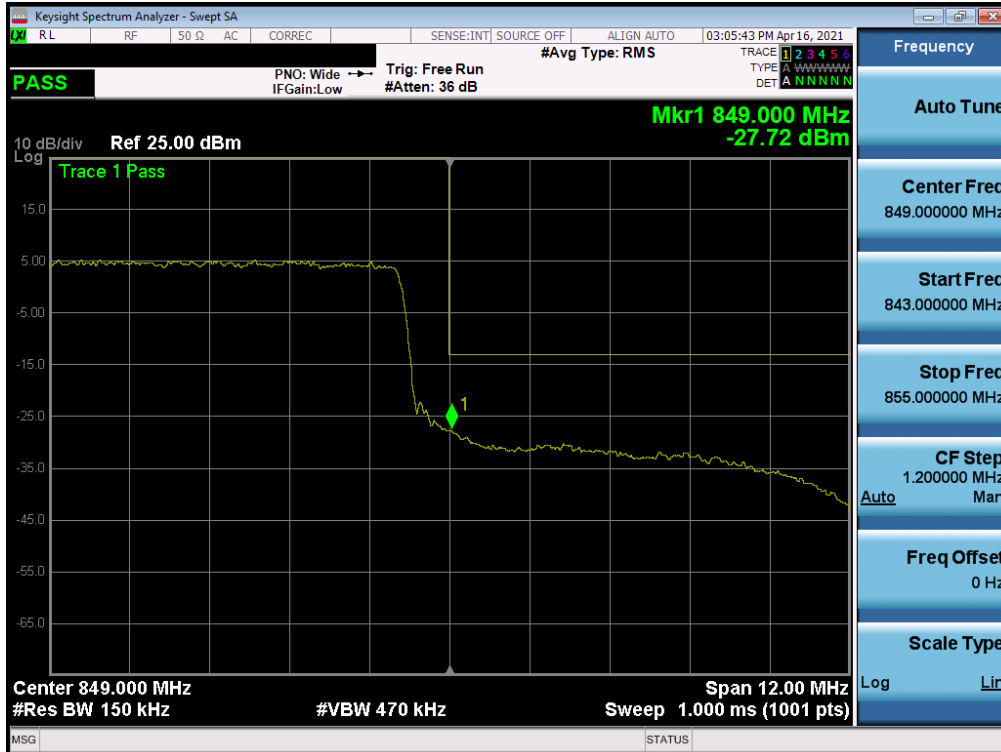
Plot 7-57. Upper Band Edge Plot (LTE Band 26 - 15MHz QPSK – Full RB)
