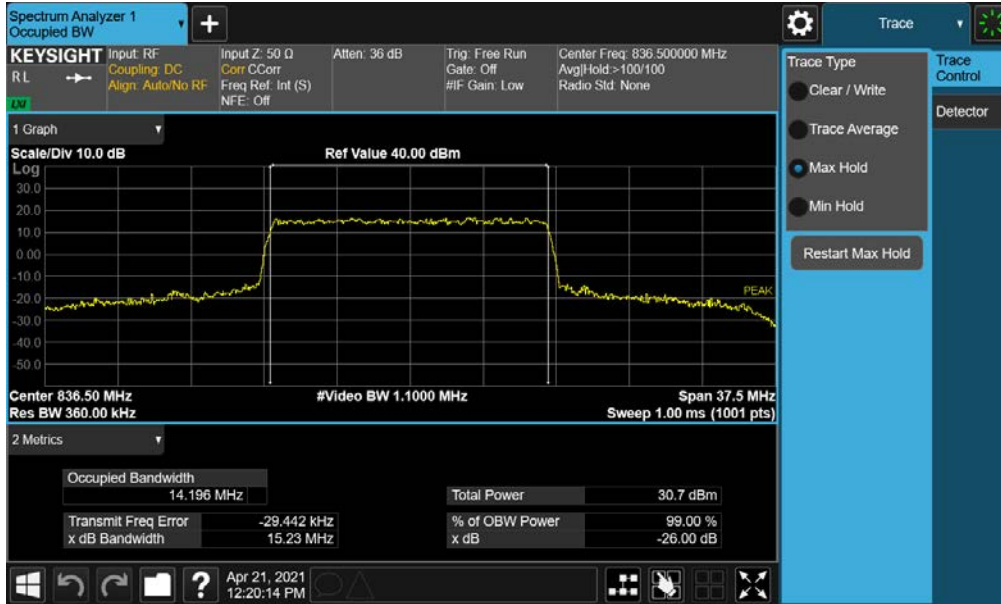
Plot 7-15. Occupied Bandwidth Plot (NR Band n5 - 15MHz QPSK - Full RB)
