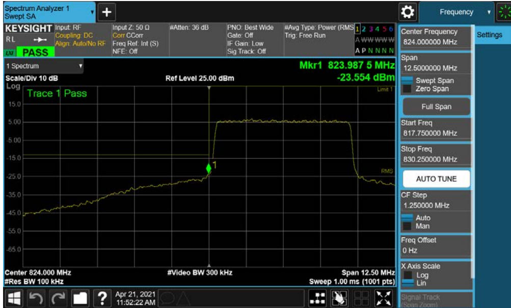
Plot 7-72. Lower Band Edge Plot (NR Band n5 – 5.0MHz - Full RB)
