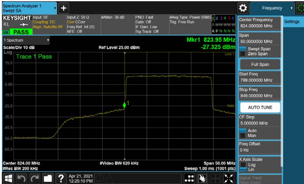
Plot 7-66. Lower Band Edge Plot (NR Band n5 – 20.0MHz - Full RB)
