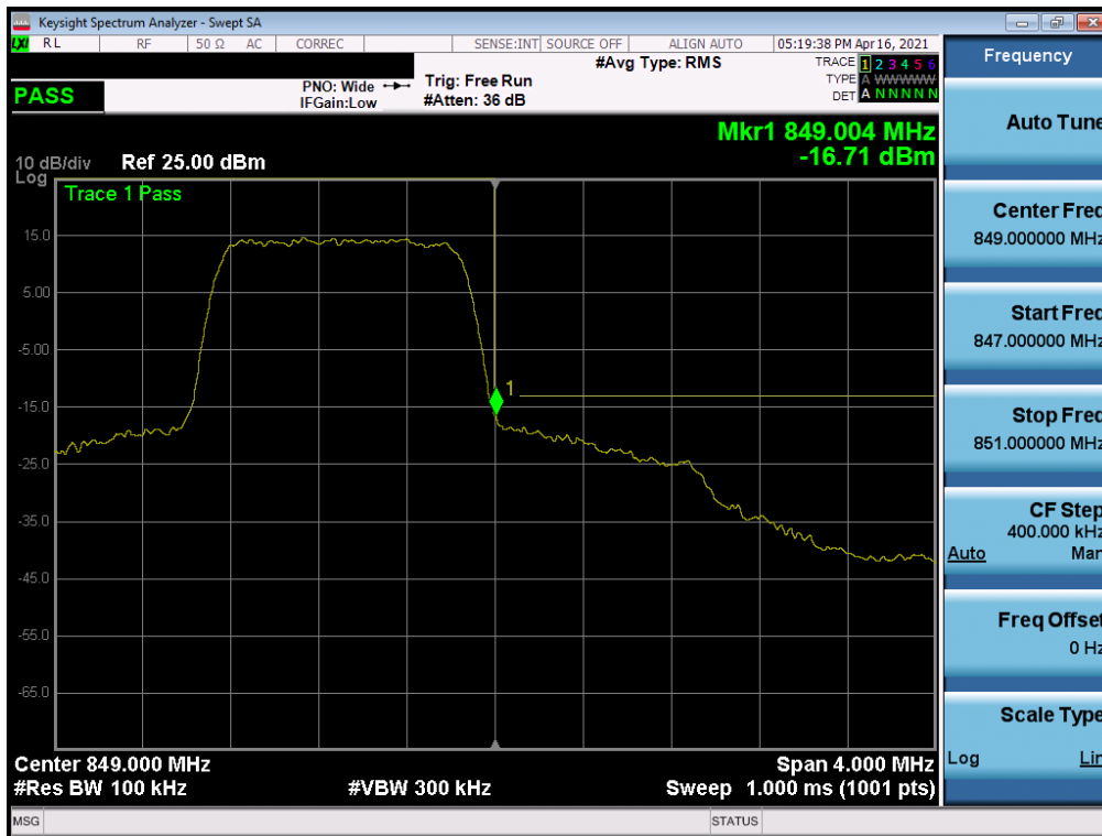
Plot 7-65. Upper Band Edge Plot (LTE Band 26/5 – 1.4MHz QPSK – Full RB)
