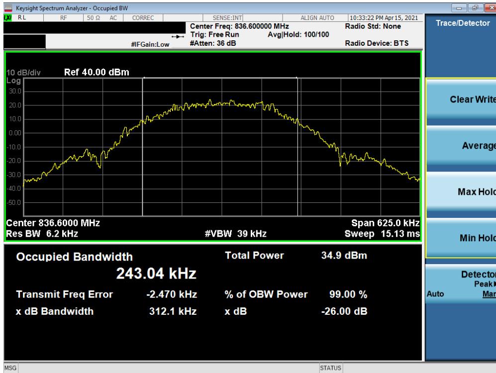
Plot 7-24. Occupied Bandwidth Plot (EDGE, Ch. 190)
