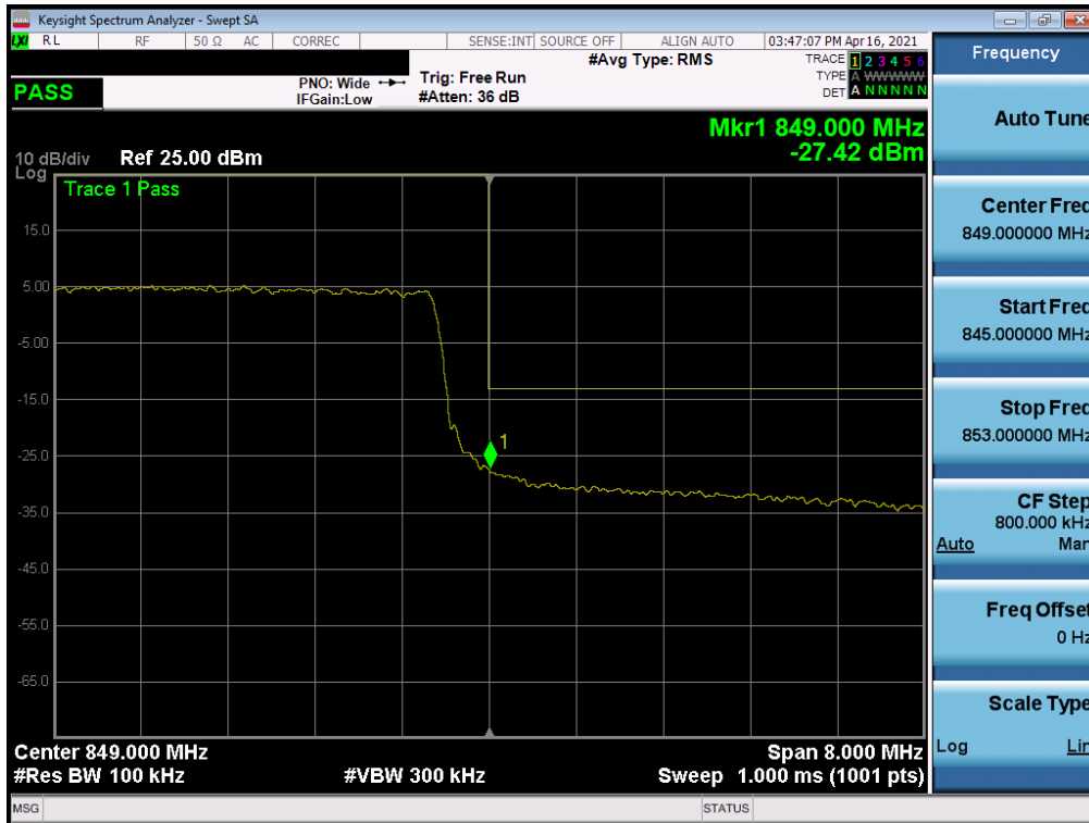
Plot 7-59. Upper Band Edge Plot (LTE Band 26/5 - 10MHz QPSK – Full RB)
