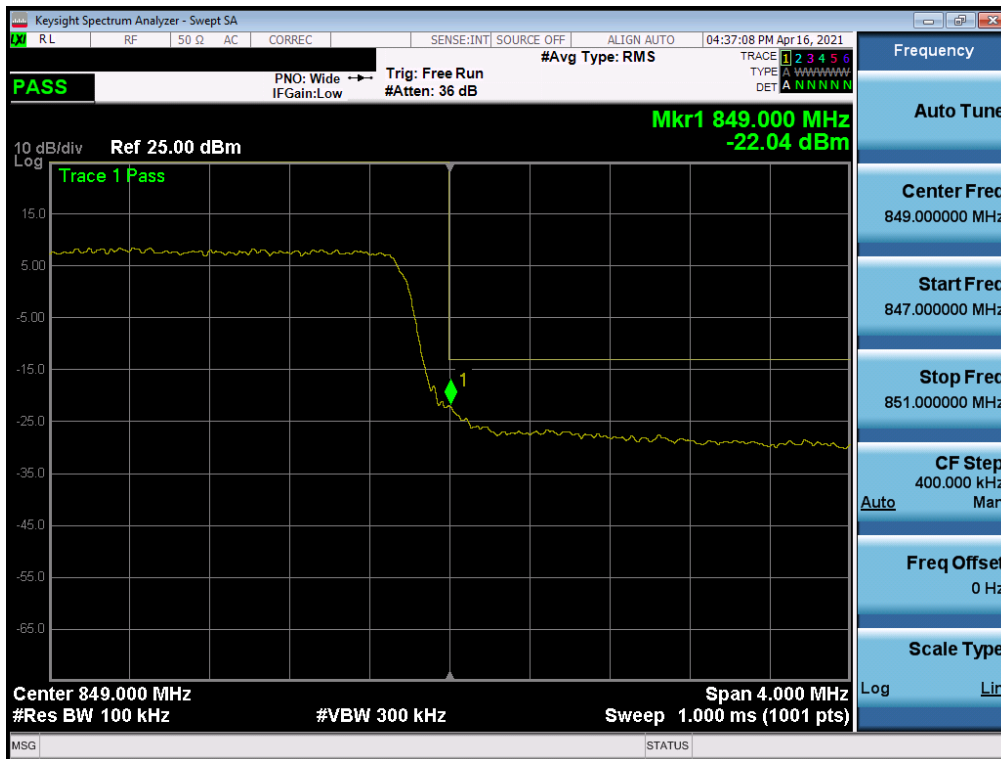
Plot 7-61. Upper Band Edge Plot (LTE Band 26/5 - 5MHz QPSK – Full RB)
