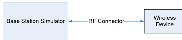
Figure 9-3 Power Measurement Setup
