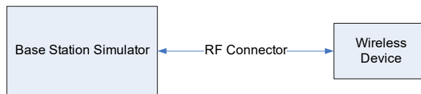
Figure 9-1 Power Measurement Setup
