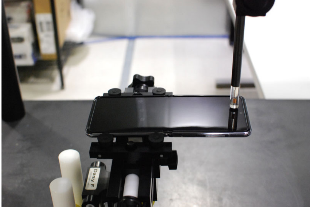
Figure 16-1 Test Setup for Wireless Device
