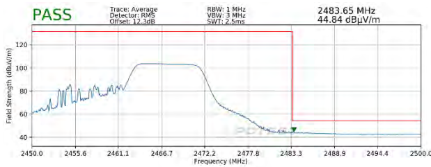
Plot 7-87. Radiated Restricted Upper Band Edge Measurement SISO ANT1 (Average – 106 Tones)
