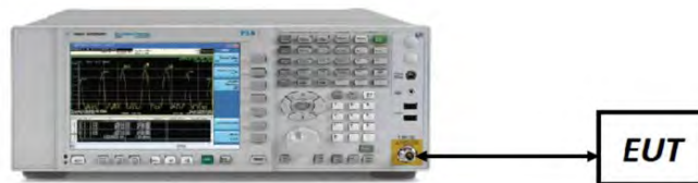
Figure 7-3. Test Instrument & Measurement Setup
