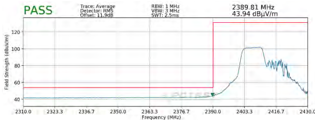
Plot 7-113. Radiated Restricted Lower Band Edge Measurement MIMO (Average – 106 Tones)
