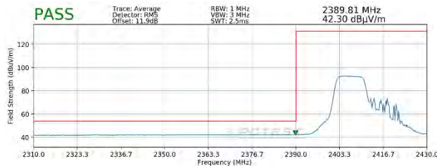
Plot 7-99. Radiated Restricted Lower Band Edge Measurement SISO ANT2 (Average – 106 Tones)
