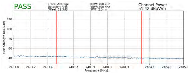
Plot 7-123. Radiated Restricted Upper Band Edge Measurement MIMO (Average – 242 Tones)
