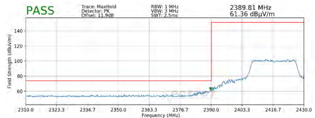
Plot 7-106. Radiated Restricted Lower Band Edge Measurement SISO ANT2 (Peak – 242 Tones)
