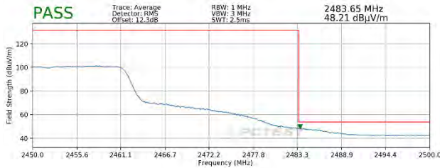
Plot 7-121. Radiated Restricted Upper Band Edge Measurement MIMO (Average – 242 Tones)
