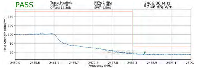
Plot 7-108. Radiated Restricted Upper Band Edge Measurement SISO ANT2 (Peak – 242 Tones)
