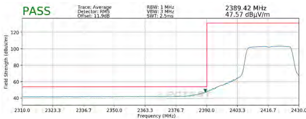
Plot 7-91. Radiated Restricted Lower Band Edge Measurement SISO ANT1 (Average – 242 Tones)
