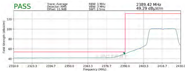
Plot 7-119. Radiated Restricted Lower Band Edge Measurement MIMO (Average – 242 Tones)
