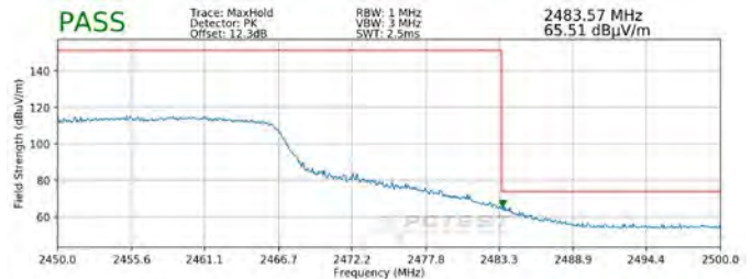
Plot 7-126. Radiated Restricted Upper Band Edge Measurement MIMO (Peak)
