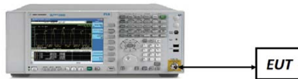
Figure 7-2. Test Instrument & Measurement Setup
