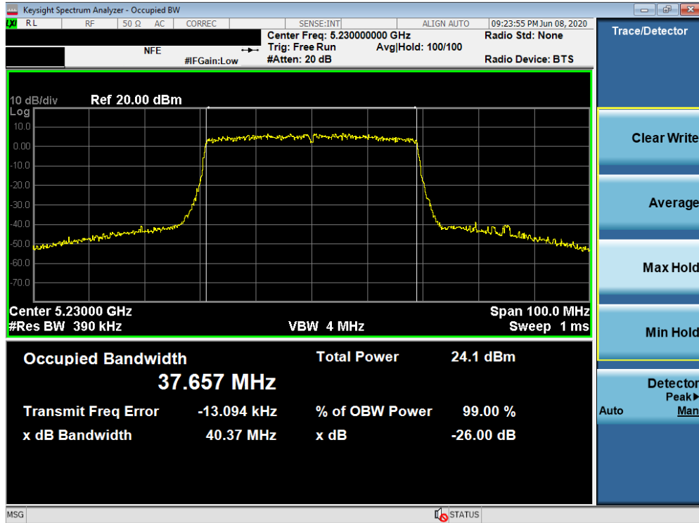
Plot 7-64. 26dB Bandwidth Plot SISO ANT2 (40MHz BW 802.11n (UNII Band 1) – Ch. 46)
