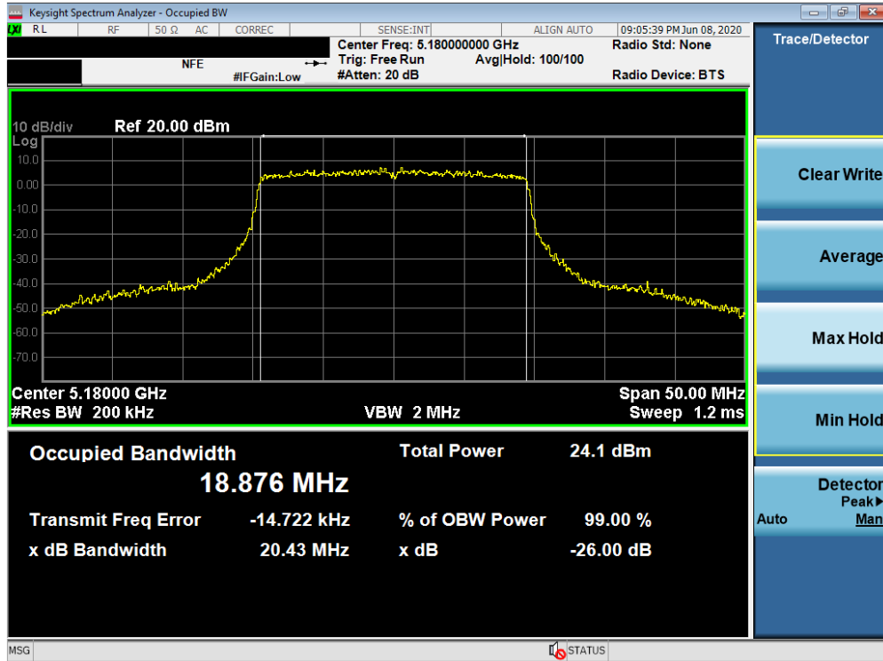
Plot 7-58. 26dB Bandwidth Plot SISO ANT2 (20MHz BW 802.11ax SU (UNII Band 1) – Ch. 36)
