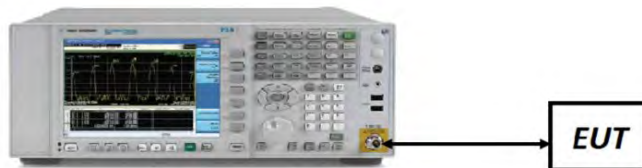
Figure 7-2. Test Instrument & Measurement Setup
