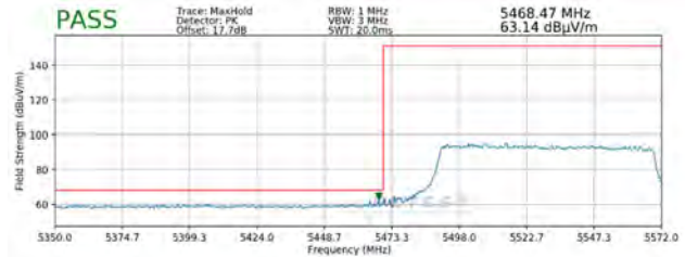
Plot 7-347. Radiated Lower Band Edge Plot SISO ANT2 (Peak – UNII Band 2C – 996 Tones)
