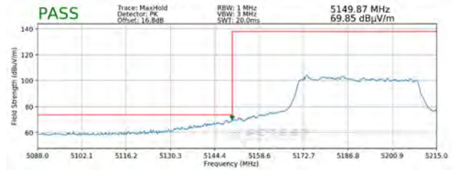
Plot 7-315. Radiated Lower Band Edge Plot SISO ANT1 (Peak – UNII Band 1 – 484 Tones)
