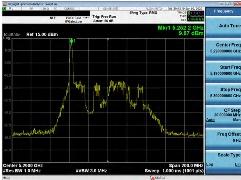
Plot 7-174. Power Spectral Density Plot SISO ANT2 (80MHz BW 802.11ax – 26 Tones (UNII Band 2A) – Ch. 58)
