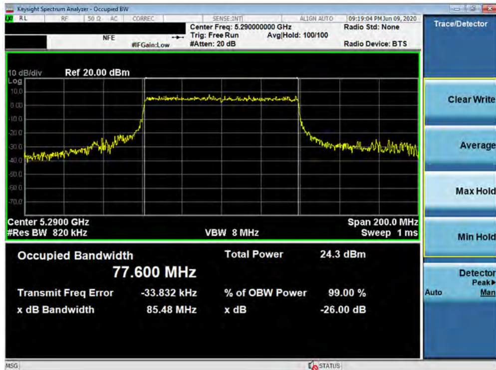
Plot 7-75. 26dB Bandwidth Plot SISO ANT2 (80MHz BW 802.11ax – 996 Tones (UNII Band 2A) – Ch. 58)
