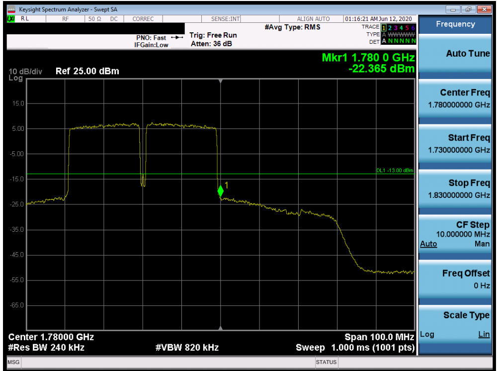
Plot 7-705. Upper Band Edge Plot (Band 66 QPSK – PCC:20 MHz SCC:20 MHz – Full RB)
