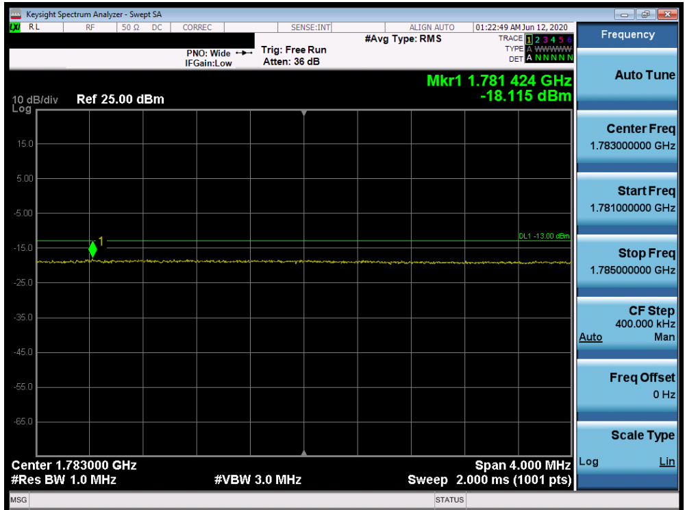
Plot 7-706. Extended Upper Band Edge Plot (Band 66 QPSK – PCC:20 MHz SCC:20 MHz – Full RB)
