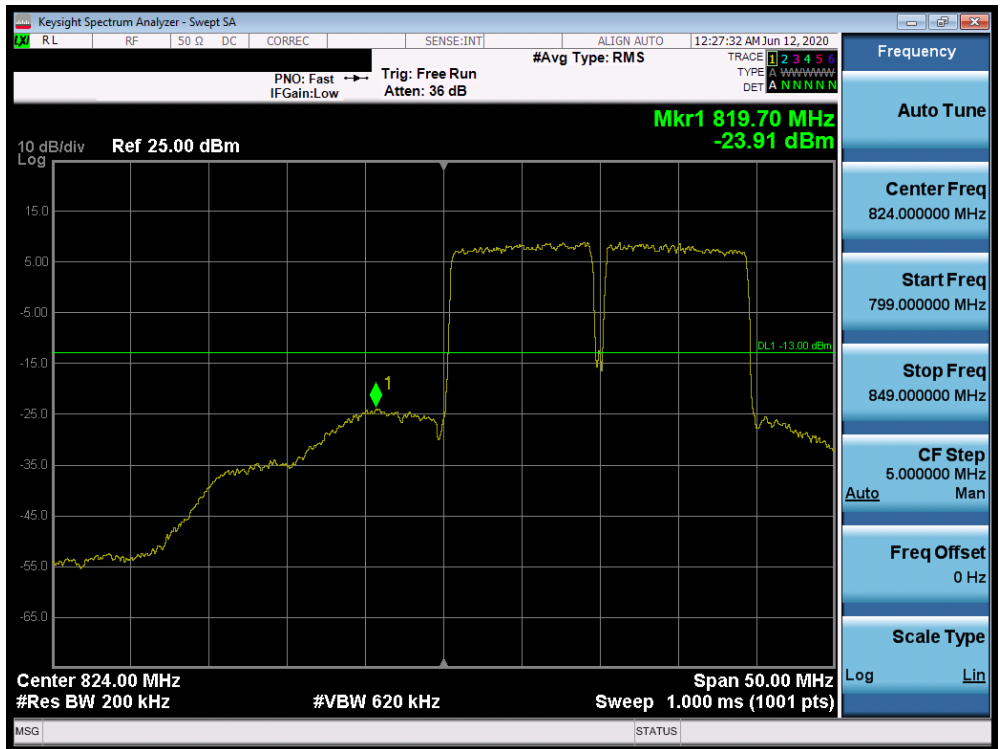
Plot 7-689. Lower Band Edge Plot (Band 5 QPSK – PCC:10 MHz SCC:10 MHz – Full RB)
