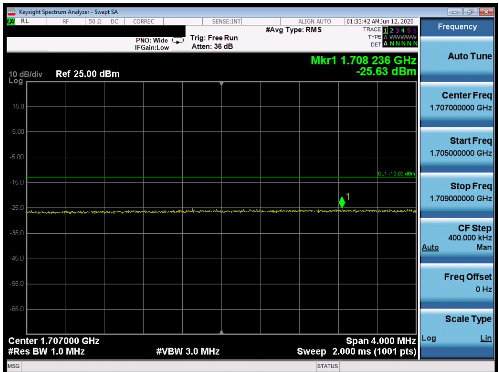
Plot 7-704. Extended Lower Band Edge Plot (Band 66 QPSK – PCC:20 MHz SCC:20 MHz – Full RB)
