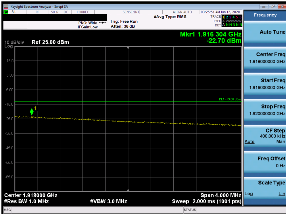
Plot 7-522. Upper Extended Band Edge Plot (Band 25 - 20.0MHz QPSK - Full RB Configuration)
