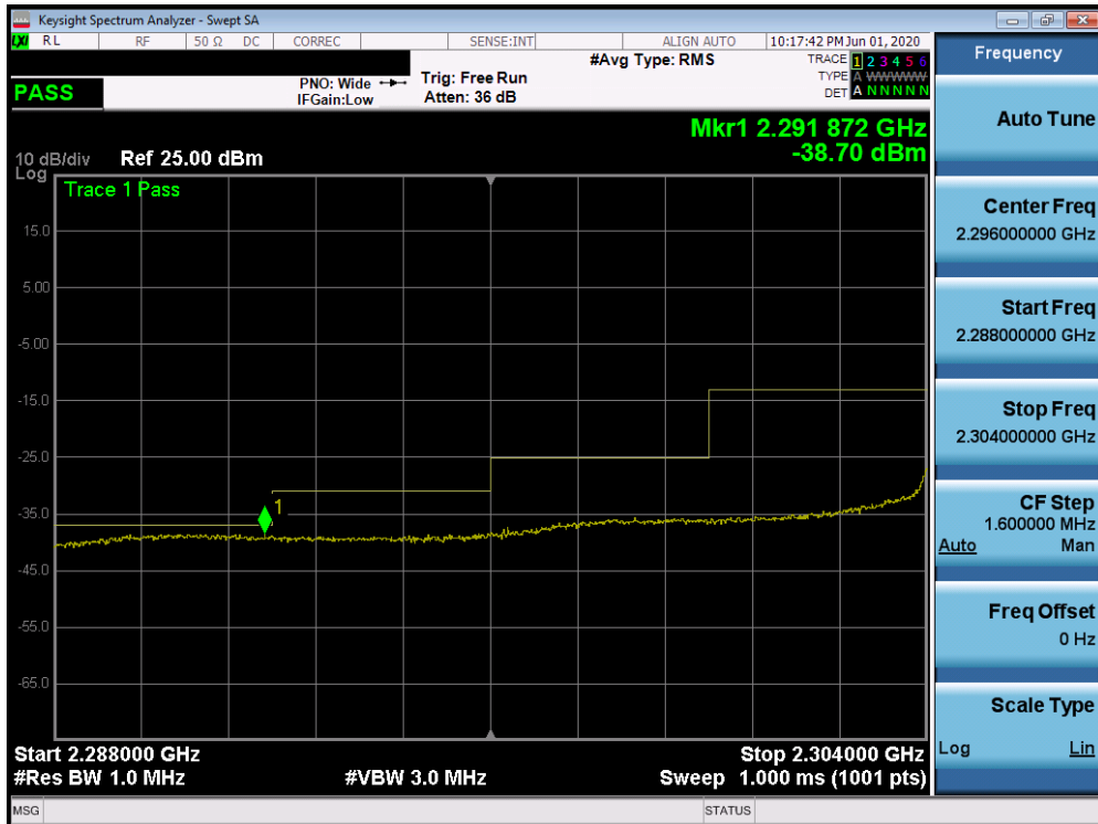
Plot 7-552. Lower Extended Band Edge Plot (Band 30 - 10.0MHz QPSK - Full RB Configuration)
