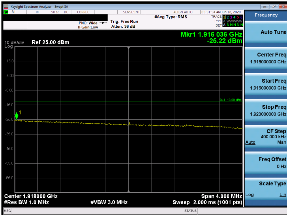
Plot 7-516. Upper Extended Band Edge Plot (Band 25 - 15.0MHz QPSK - Full RB Configuration)
