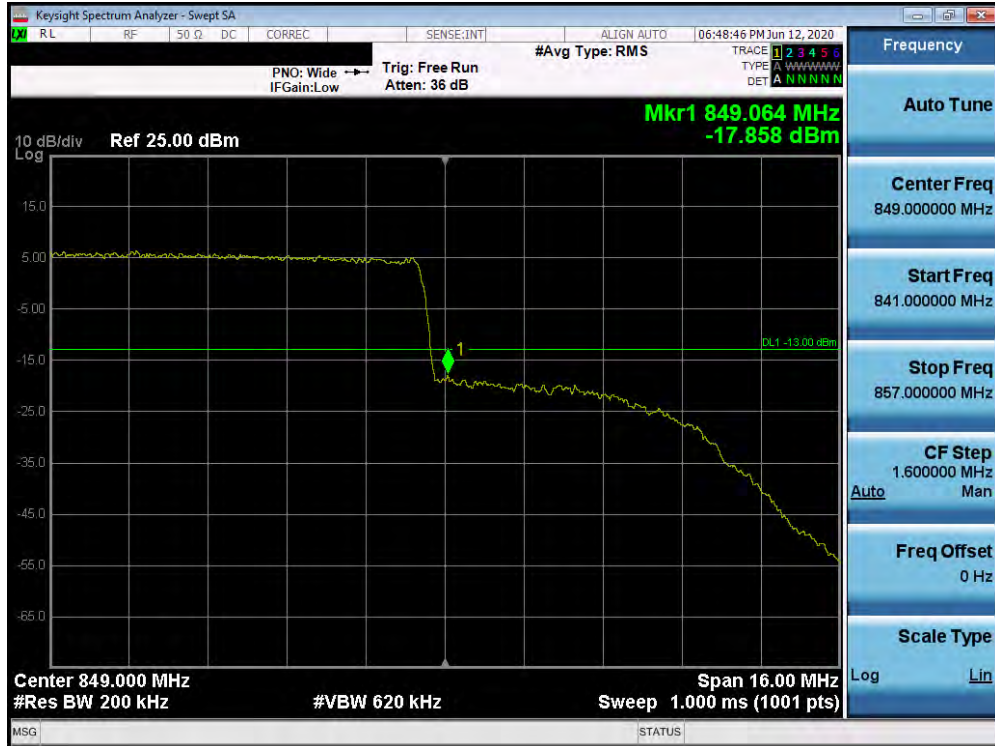
Plot 7-434. Upper Band Edge Plot (n5 – 20.0MHz DFT-s-OFDM BPSK - Full RB Configuration)
