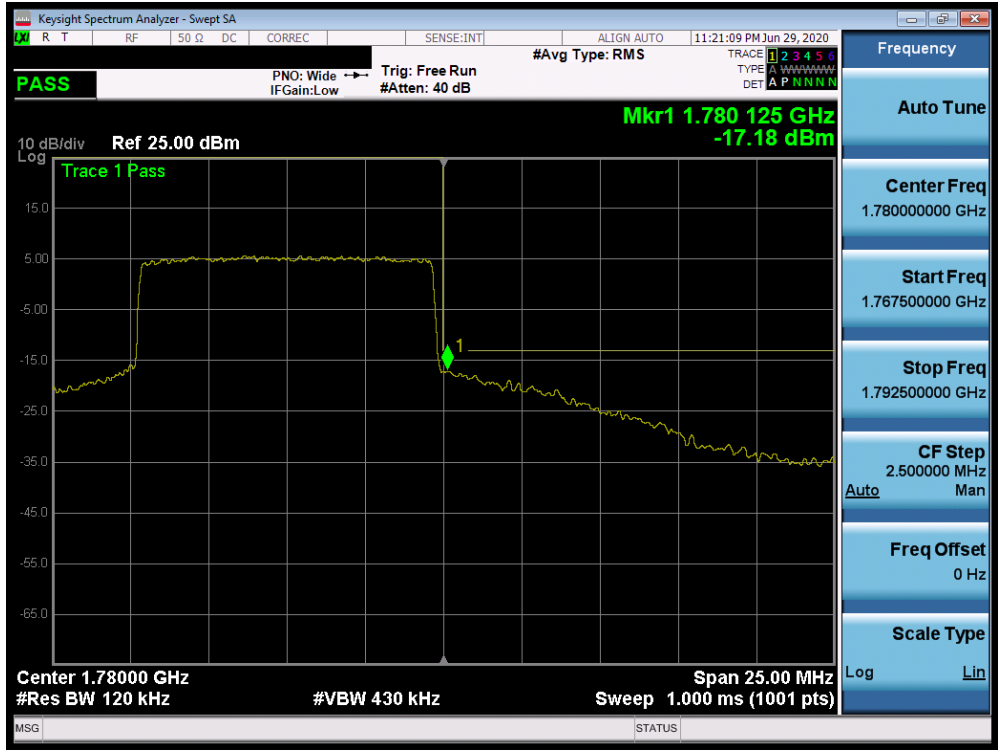
Plot 7-477. Upper Band Edge Plot (n66 - 10MHz DFT-s-OFDM-QPSK - Full RB Configuration)
