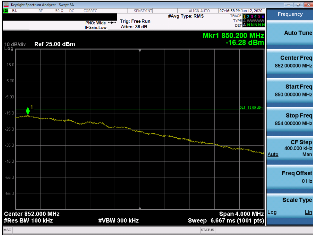
Plot 7-428. Upper Extended Band Edge Plot (n5 – 5.0MHz DFT-s-OFDM BPSK - Full RB Configuration)
