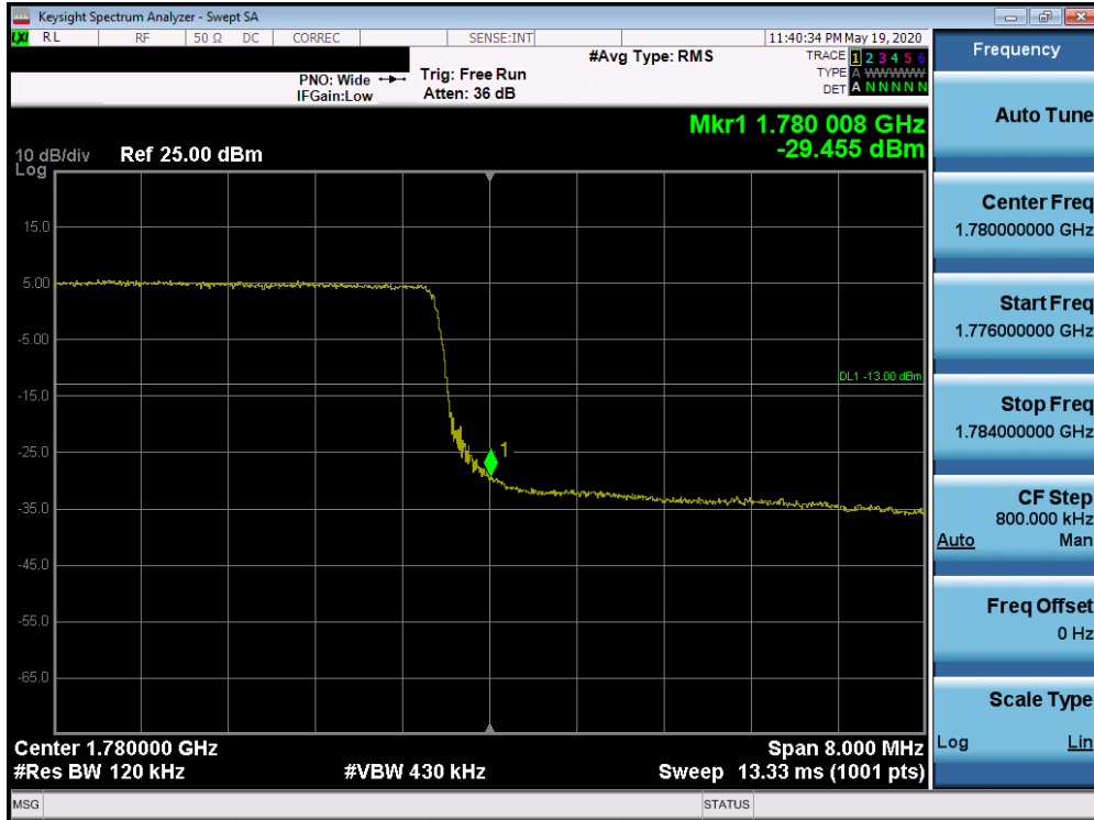
Plot 7-457. Upper Band Edge Plot (Band 66 - 10.0MHz QPSK - Full RB Configuration)
