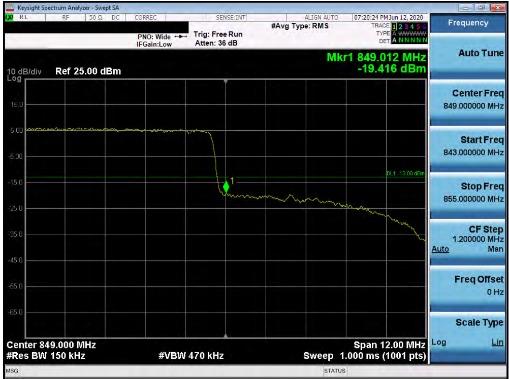
Plot 7-432. Upper Band Edge Plot (n5 – 15.0MHz DFT-s-OFDM BPSK - Full RB Configuration)
