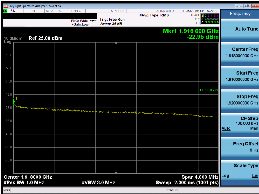
Plot 7-510. Upper Extended Band Edge Plot (Band 25 - 10.0MHz QPSK - Full RB Configuration)
