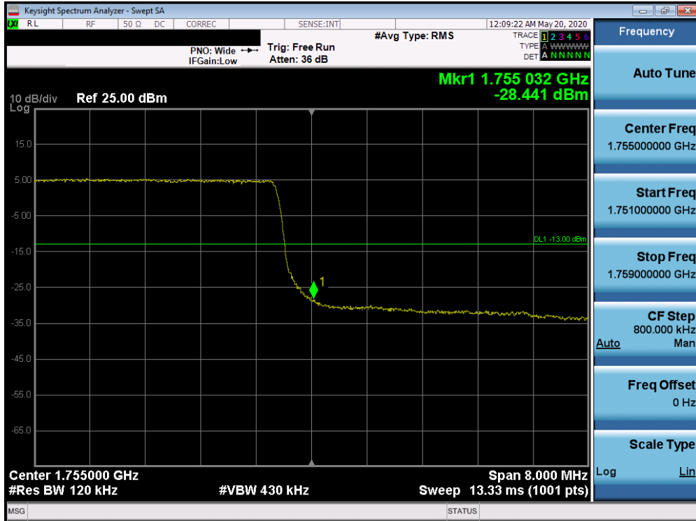
Plot 7-455. Upper Band Edge Plot (Band 4 - 10.0MHz QPSK - Full RB Configuration)
