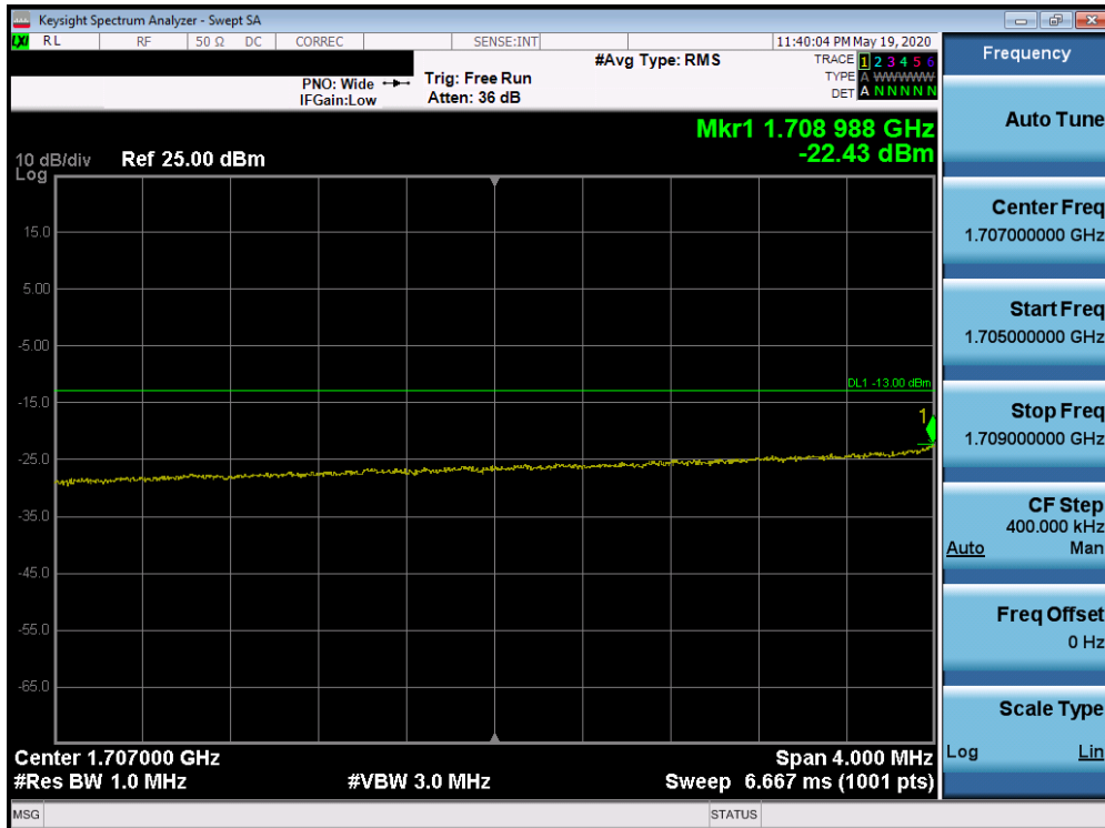
Plot 7-454. Lower Extended Band Edge Plot (Band 66/4 - 10.0MHz QPSK - Full RB Configuration)
