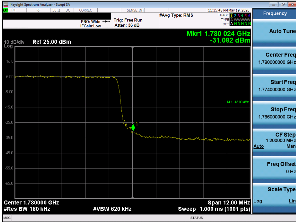
Plot 7-463. Upper Band Edge Plot (Band 66 - 15.0MHz QPSK - Full RB Configuration)
