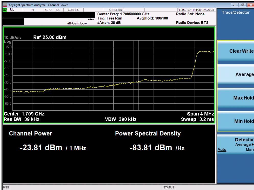
Plot 7-436. Lower Extended Band Edge Plot (Band 66/4 - 1.4MHz QPSK - Full RB Configuration)
