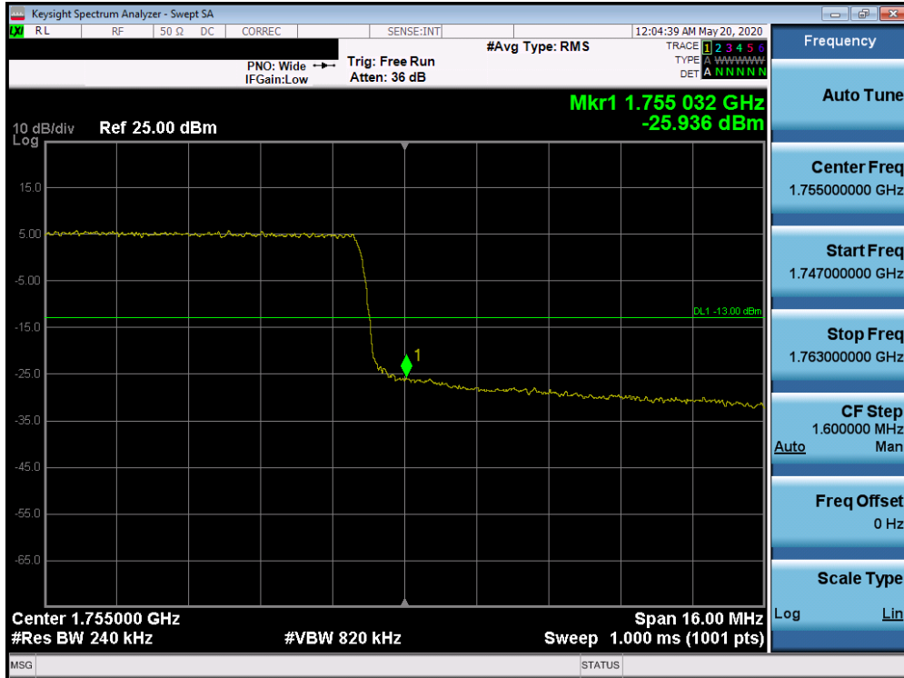
Plot 7-467. Upper Band Edge Plot (Band 4 - 20.0MHz QPSK - Full RB Configuration)
