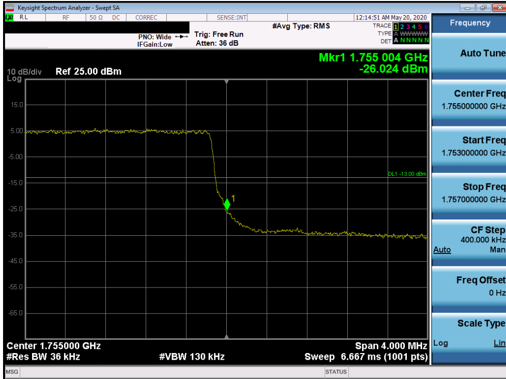
Plot 7-443. Upper Band Edge Plot (Band 4 - 3.0MHz QPSK - Full RB Configuration)
