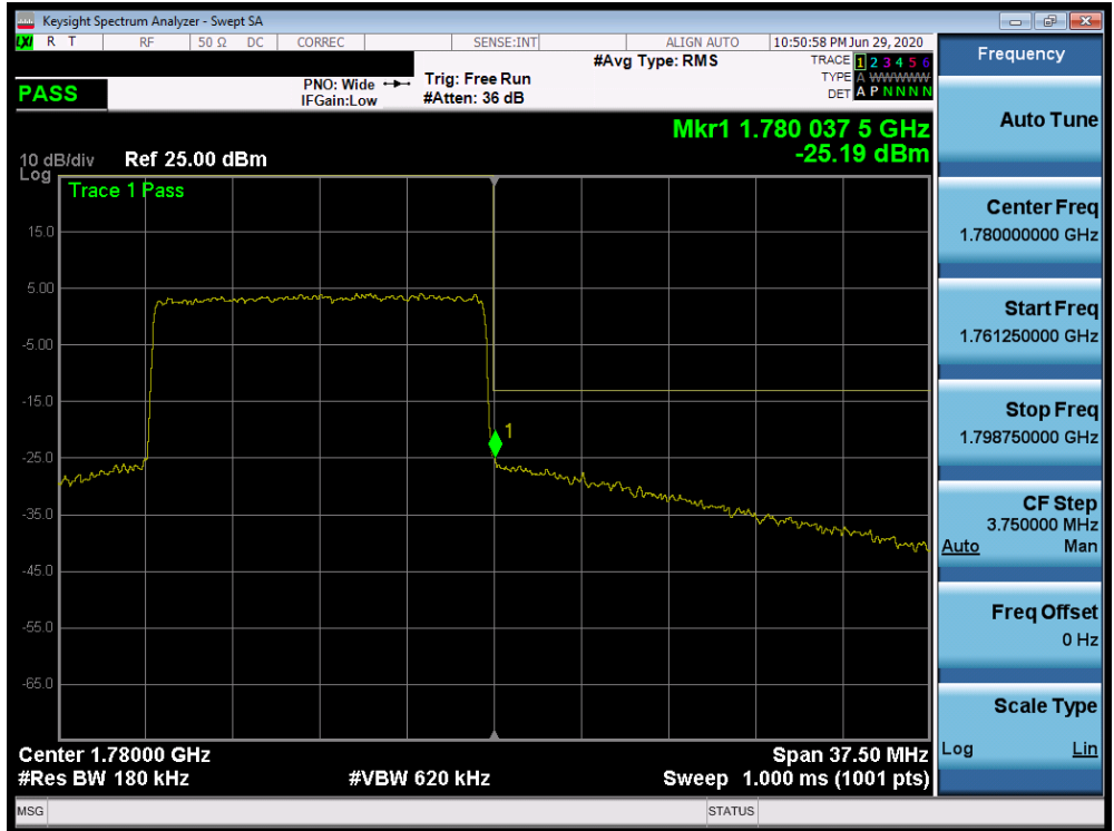
Plot 7-481. Upper Band Edge Plot (n66 - 15MHz DFT-s-OFDM-QPSK - Full RB Configuration)
