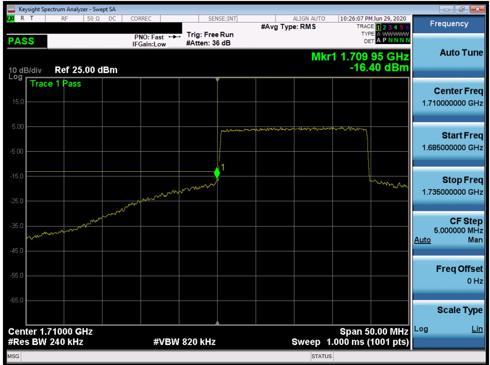
Plot 7-483. Lower Band Edge Plot (n66 - 20MHz DFT-s-OFDM-QPSK - Full RB Configuration)
