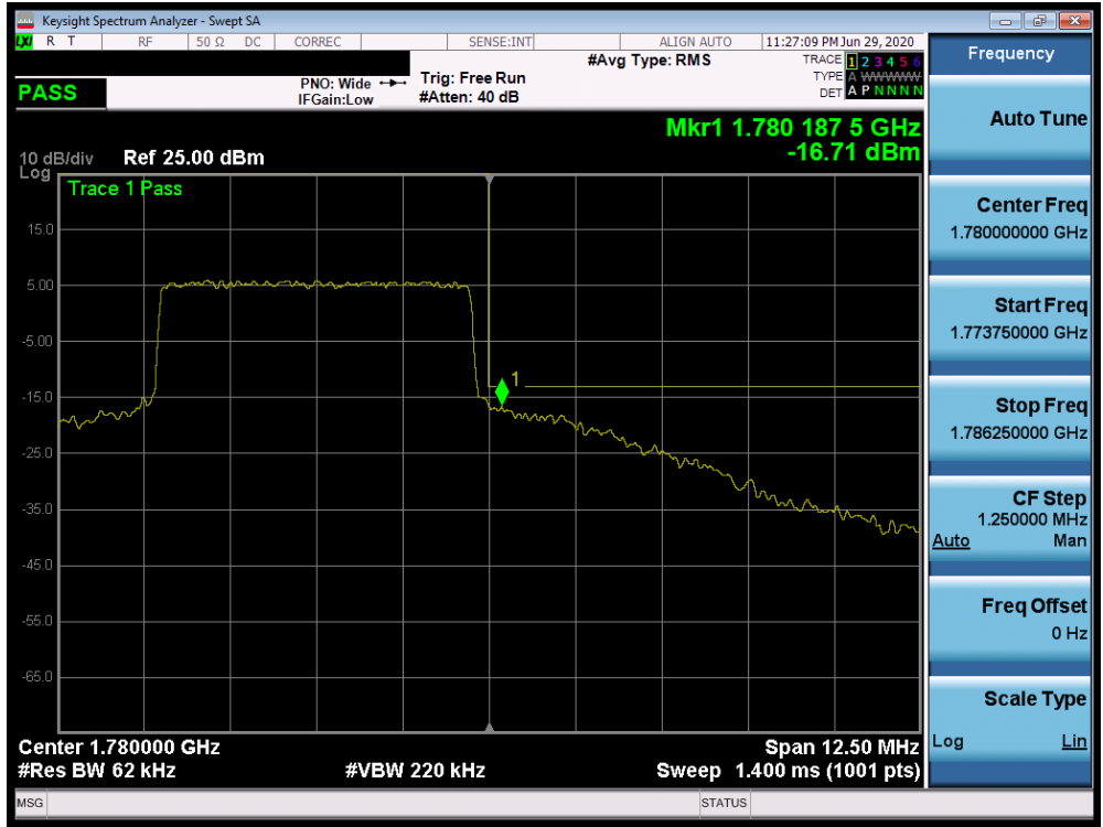
Plot 7-473. Upper Band Edge Plot (n66 - 5MHz DFT-s-OFDM-QPSK - Full RB Configuration)
