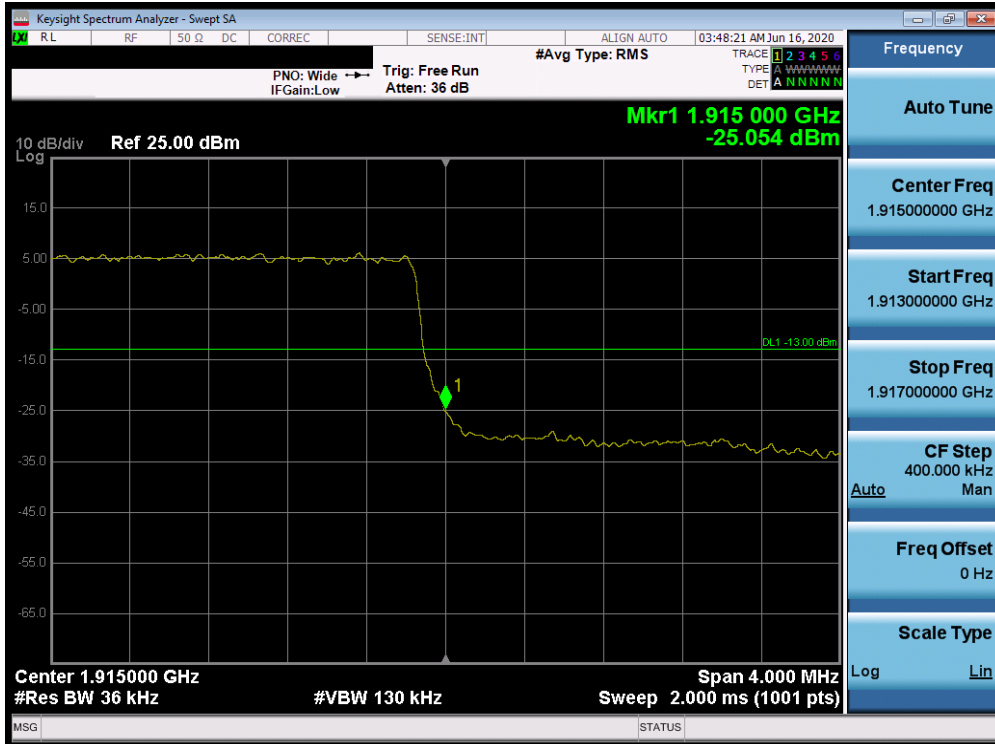
Plot 7-497. Upper Band Edge Plot (Band 25 - 3.0MHz QPSK - Full RB Configuration)
