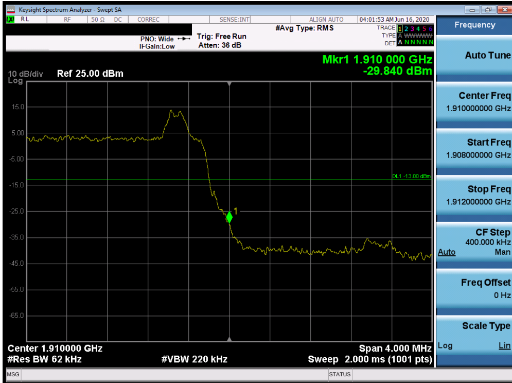
Plot 7-501. Upper Band Edge Plot (Band 2 - 5.0MHz QPSK - Full RB Configuration)
