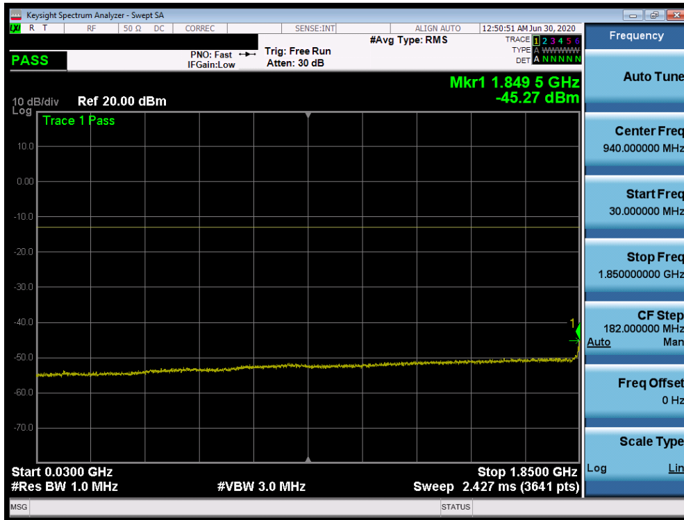
Plot 7-339. Conducted Spurious Plot (n25/2 - 20MHz DFT-s-OFDM-QPSK - RB Size 1, RB Offset 1 - Low Channel)
