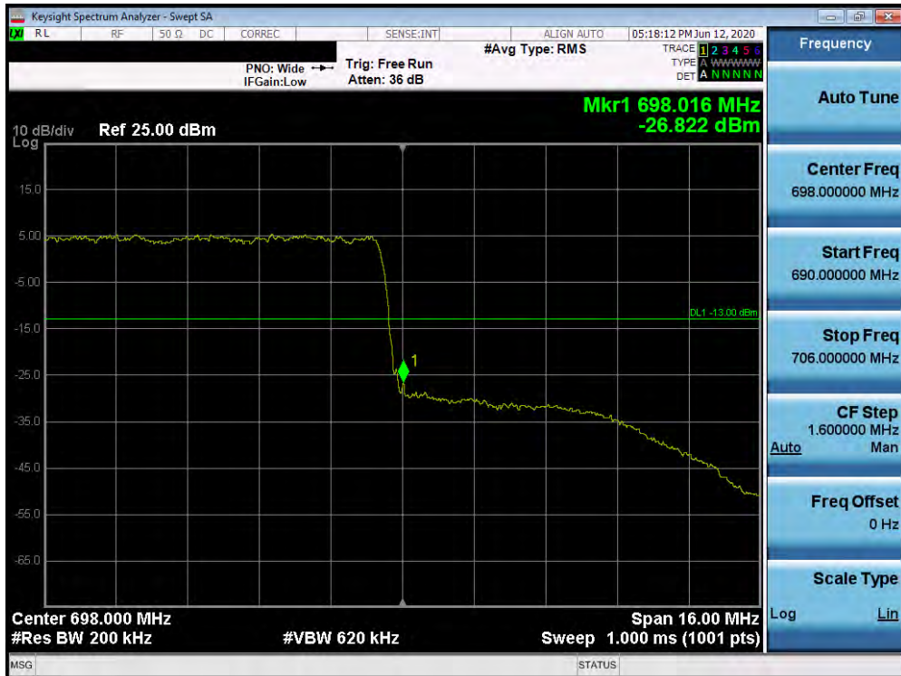
Plot 7-399. Upper Band Edge Plot (n71- 20MHz DFT-s-OFDM-QPSK - Full RB Configuration)
