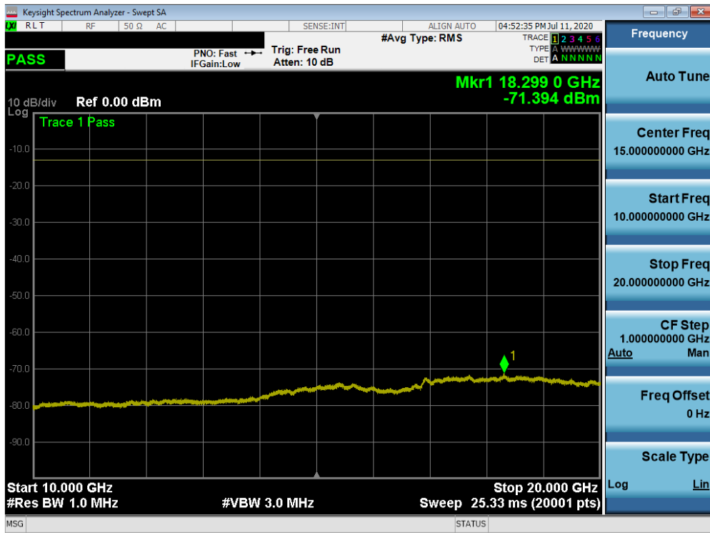
Plot 7-347. Conducted Spurious Plot (n25/2 - 20MHz DFT-s-OFDM-QPSK - RB Size 1, RB Offset 1 - High Channel)
