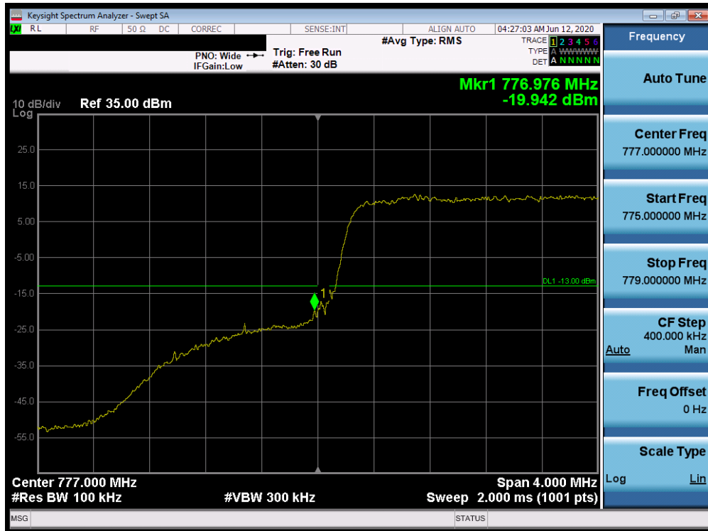
Plot 7-408. Lower Band Edge Plot (Band 13 - 5.0MHz QPSK - Full RB Configuration)
