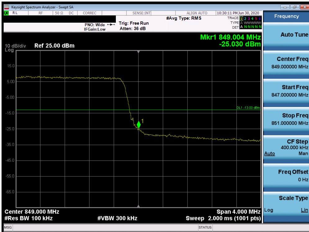
Plot 7-421. Upper Band Edge Plot (Band 26/5 - 5.0MHz QPSK - Full RB Configuration)
