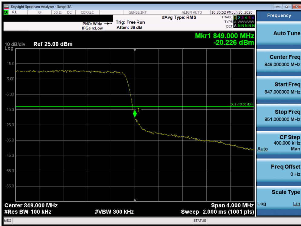
Plot 7-419. Upper Band Edge Plot (Band 26/5 - 3.0MHz QPSK - Full RB Configuration)
