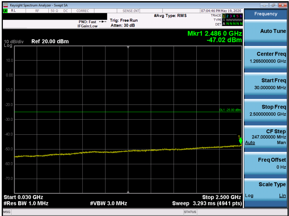
Plot 7-360. Conducted Spurious Plot (Band 7 - 20.0MHz QPSK - RB Size 1, RB Offset 0 - Mid Channel)
