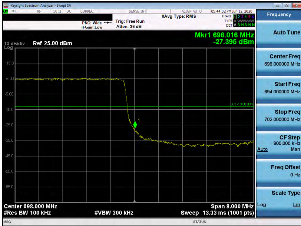
Plot 7-395. Upper Band Edge Plot (n71 - 10MHz DFT-s-OFDM-QPSK - Full RB Configuration)
