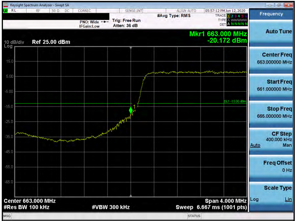
Plot 7-392. Lower Band Edge Plot (n71 - 5MHz DFT-s-OFDM-QPSK - Full RB Configuration)
