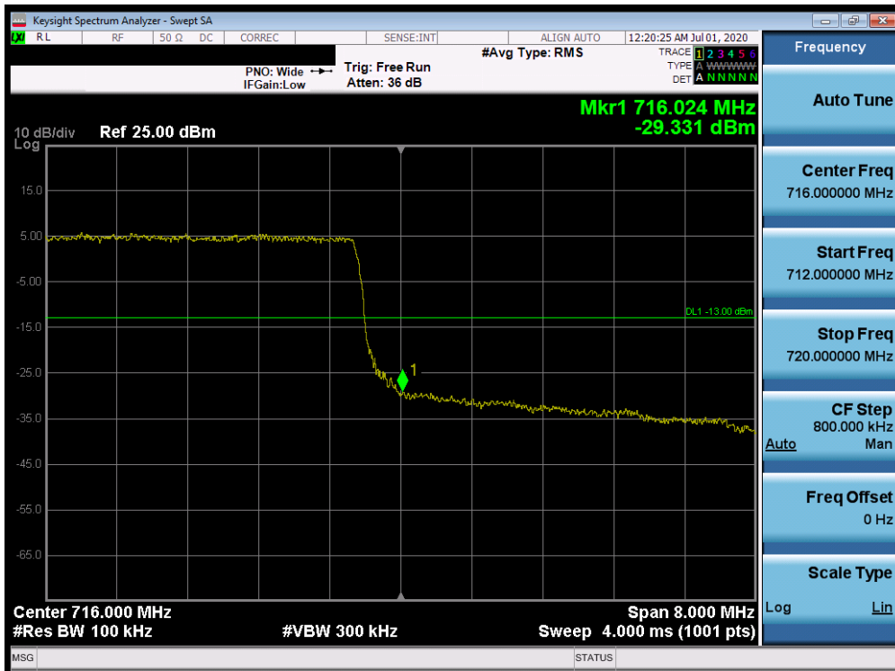
Plot 7-407. Upper Band Edge Plot (Band 12 - 10.0MHz QPSK - Full RB Configuration)
