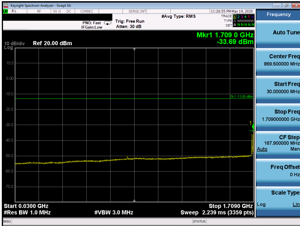
Plot 7-312. Conducted Spurious Plot (Band 66/4 - 20.0MHz QPSK - RB Size 1, RB Offset 0 - Low Channel)
