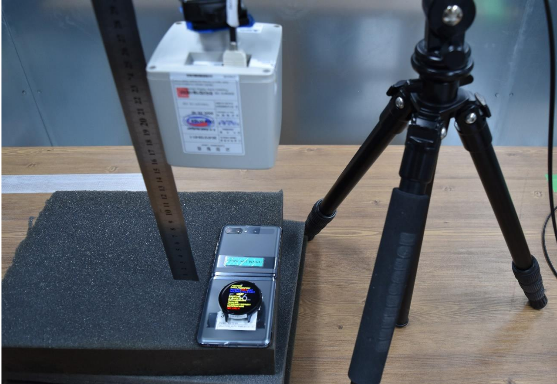
Top – charger below client (20cm distance)
