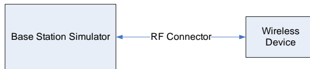
Figure 9-1 Power Measurement Setup
