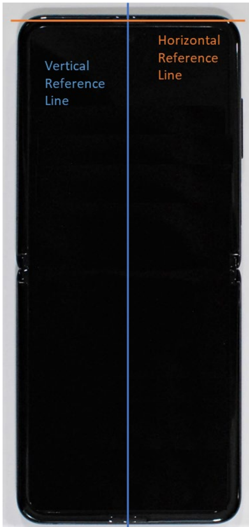
SAR Test Setup Photo 21 – Vertical and Horizontal Reference Lines
