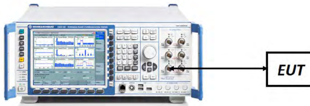
Figure 7-8. ERP/EIRP Measurement Setup
