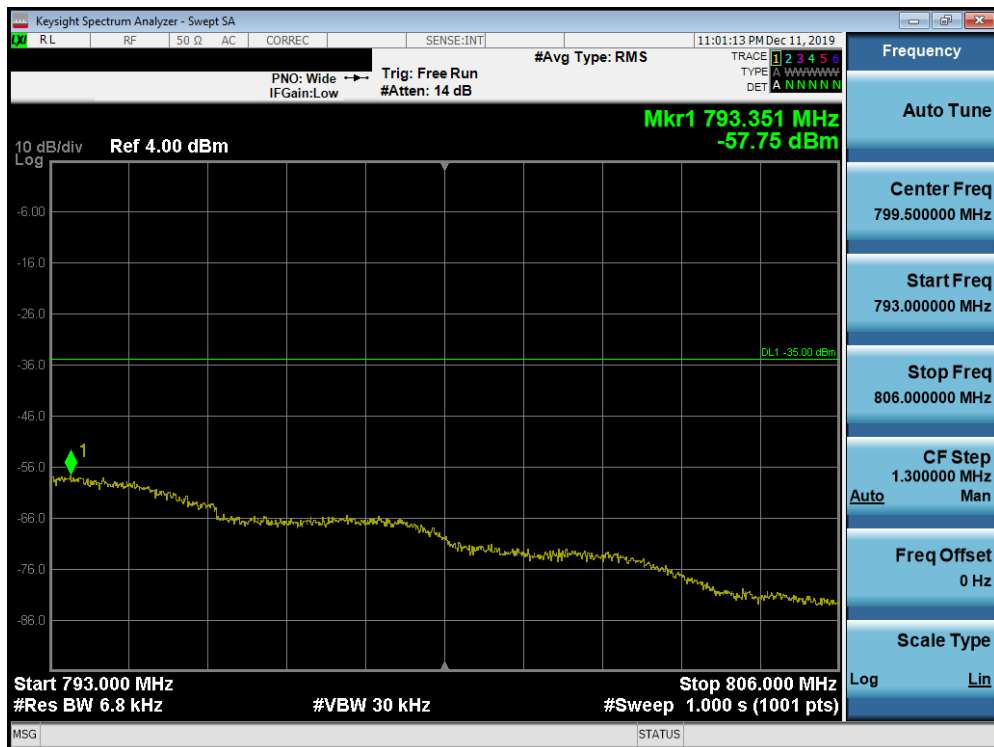
Plot 7-152. Upper Emission Mask Plot (Band 13 - 5.0MHz QPSK - Full RB Configuration)
