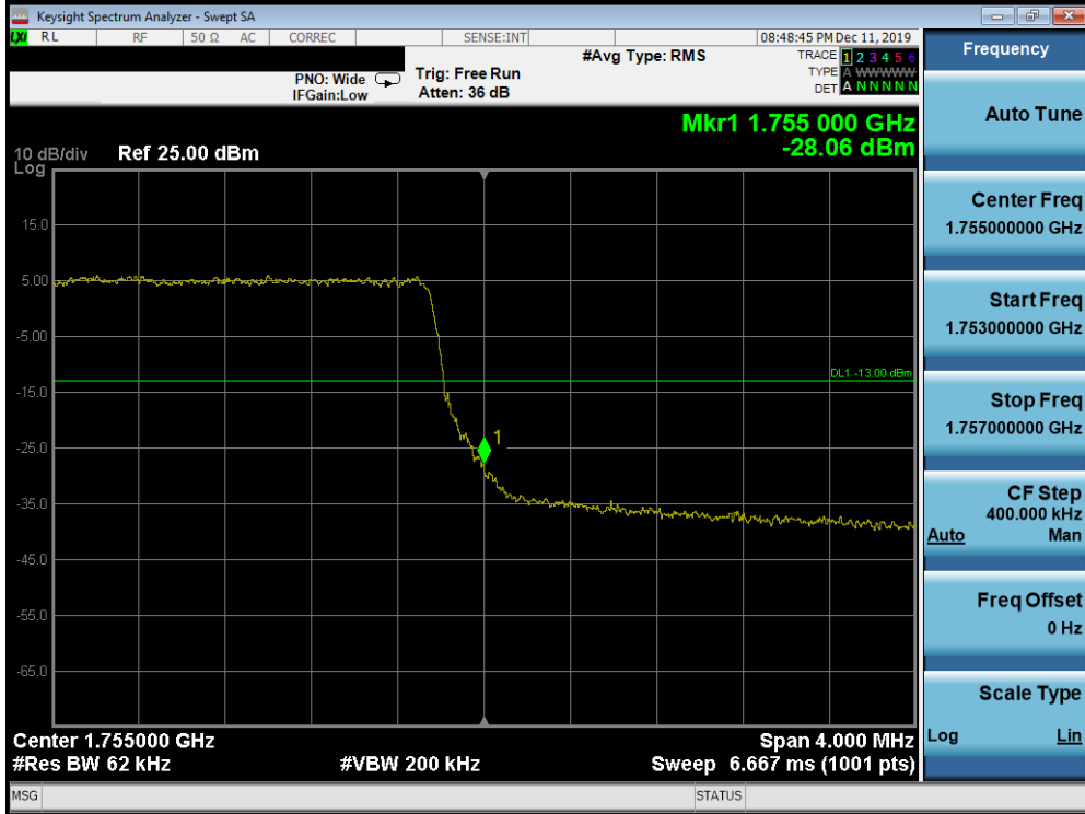
Plot 7-181. Upper Band Edge Plot (Band 4 – 5.0MHz QPSK - Full RB Configuration)
