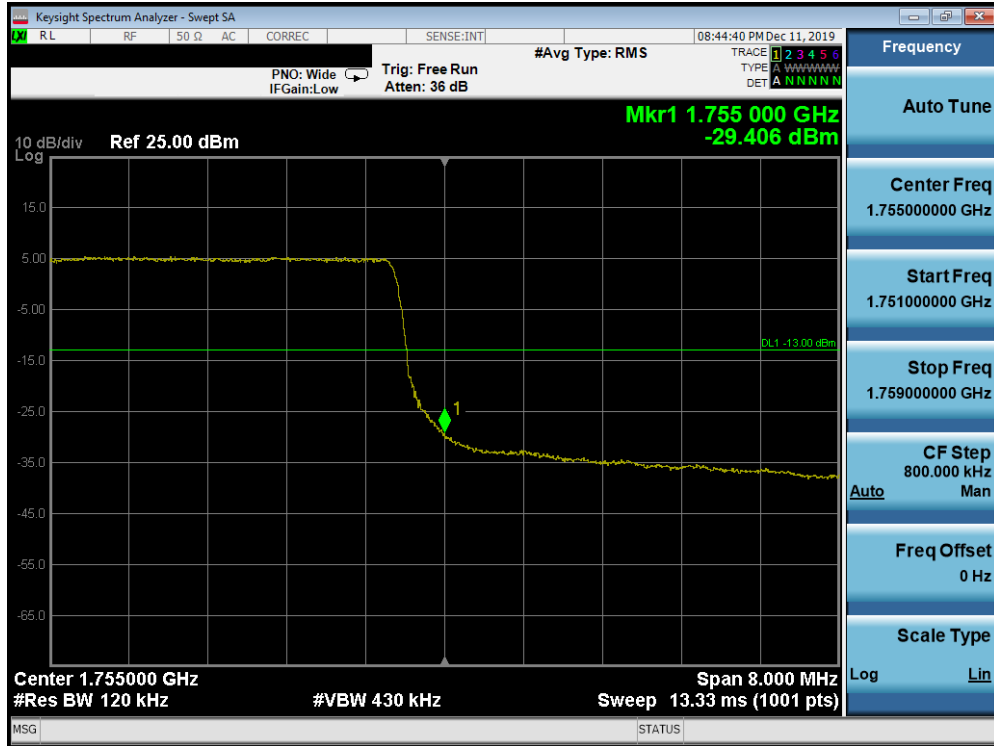
Plot 7-187. Upper Band Edge Plot (Band 4 – 10.0MHz QPSK - Full RB Configuration)
