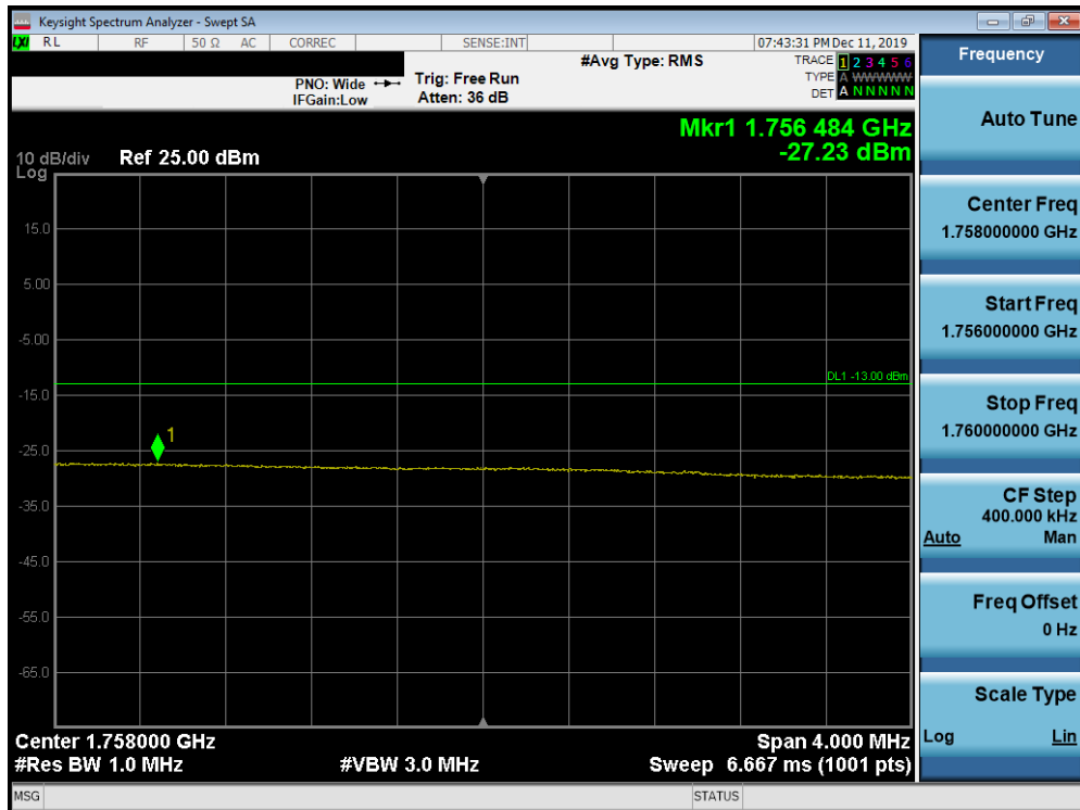
Plot 7-200. Upper Extended Band Edge Plot (Band 4 – 20.0MHz QPSK - Full RB Configuration)
