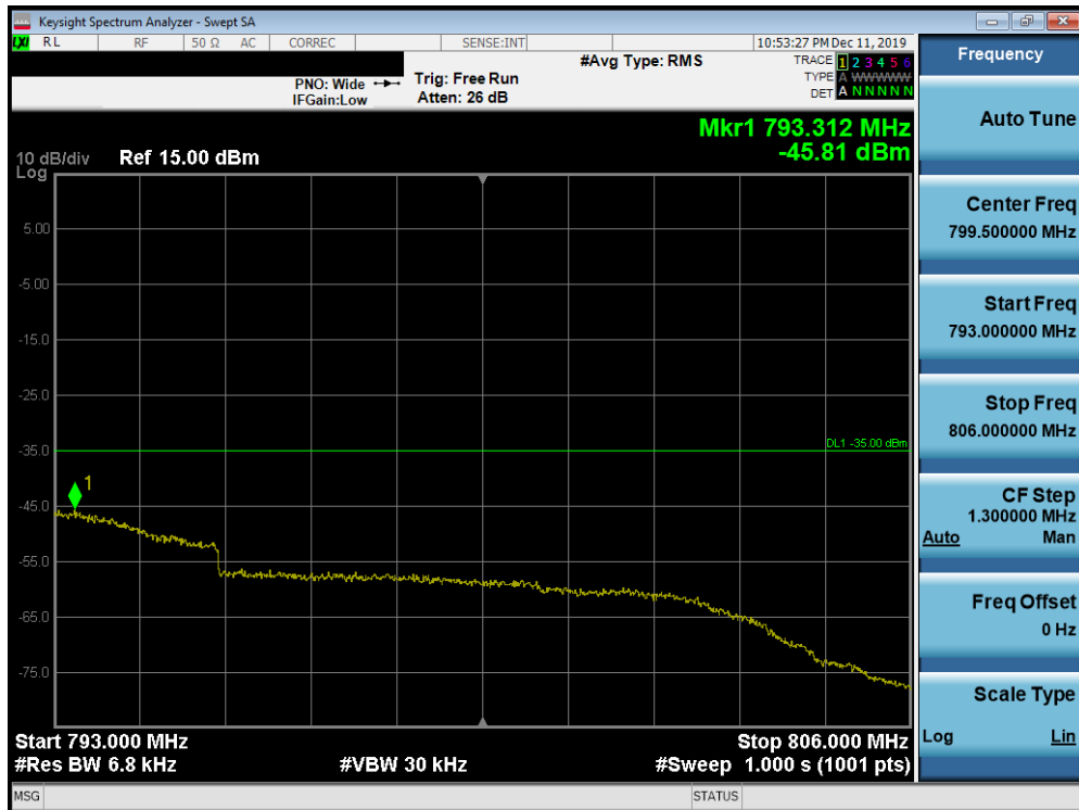
Plot 7-156. Upper Emission Mask Plot (Band 13 - 10.0MHz QPSK - Full RB Configuration)
