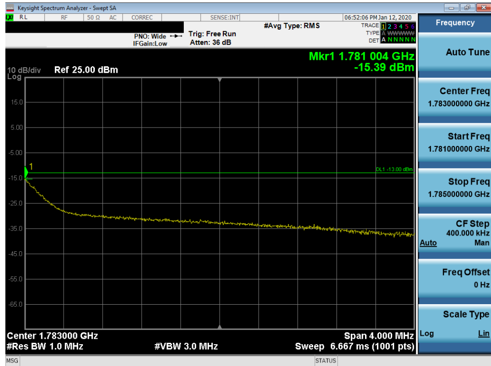
Plot 7-184. Upper Extended Band Edge Plot (Band 66 - 5.0MHz QPSK - Full RB Configuration)
