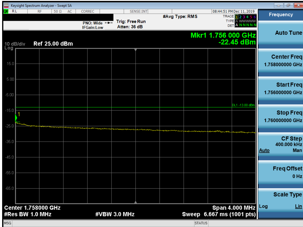
Plot 7-188. Upper Extended Band Edge Plot (Band 4 – 10.0MHz QPSK - Full RB Configuration)
