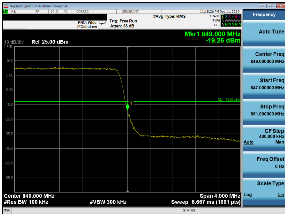
Plot 7-160. Upper Band Edge Plot (Band 26/5 - 3.0MHz QPSK - Full RB Configuration)
