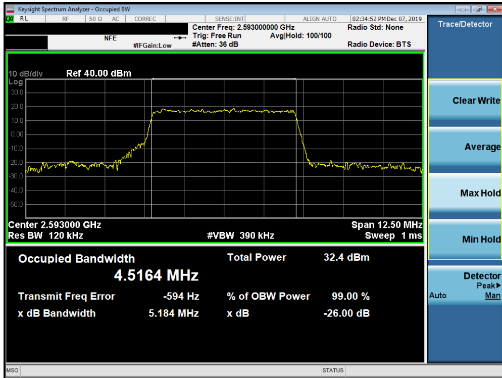
Plot 7-76. Occupied Bandwidth Plot (Band 41 PC3 - 5.0MHz QPSK - Full RB Configuration)
