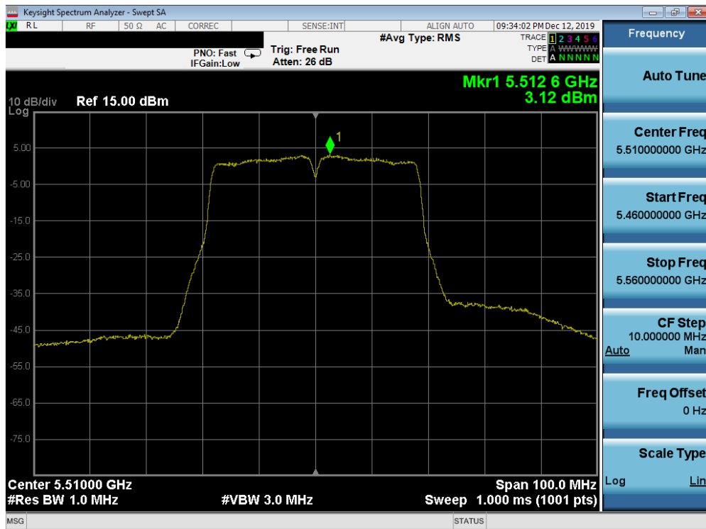
Plot 7-142. Power Spectral Density Plot SISO ANT2 (40MHz BW 802.11n (UNII Band 2C) – Ch. 102)
