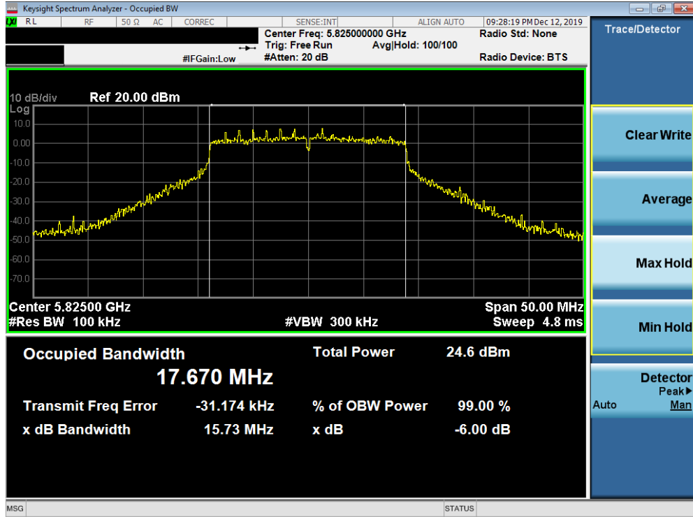
Plot 7-75. 6dB Bandwidth Plot SISO ANT2 (20MHz BW 802.11n (UNII Band 3) – Ch. 165)
