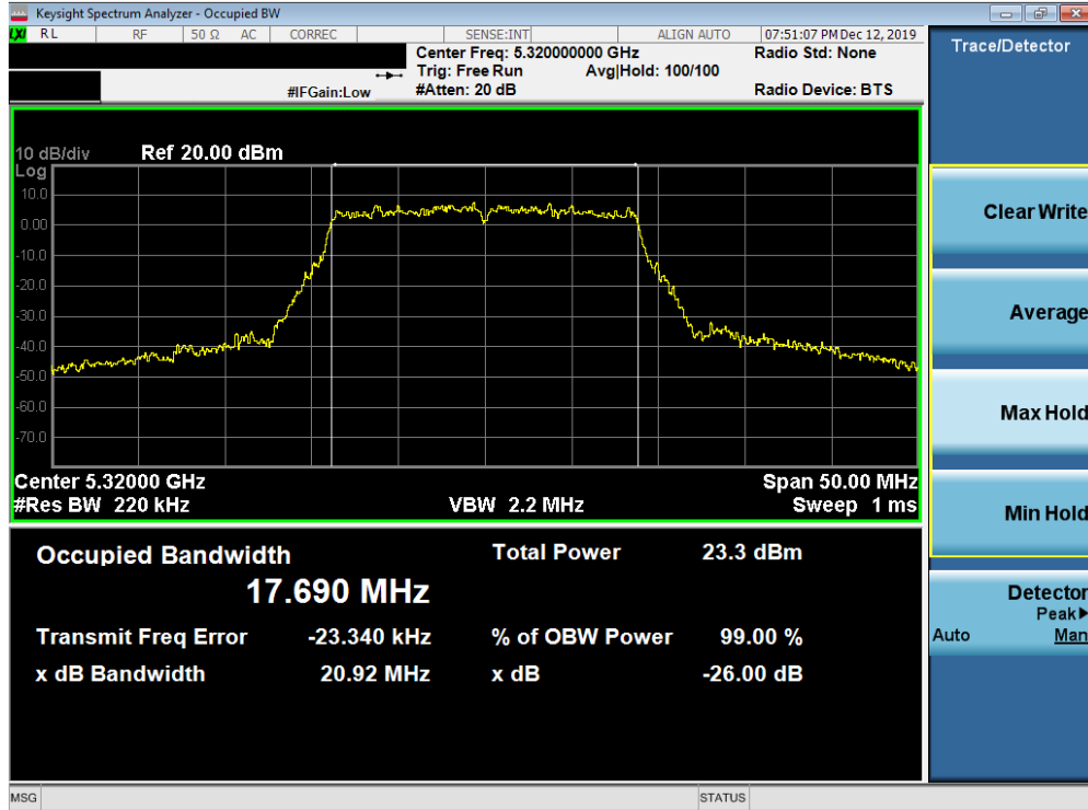
Plot 7-15. 26dB Bandwidth Plot SISO ANT1 (20MHz BW 802.11n (UNII Band 2A) – Ch. 64)
