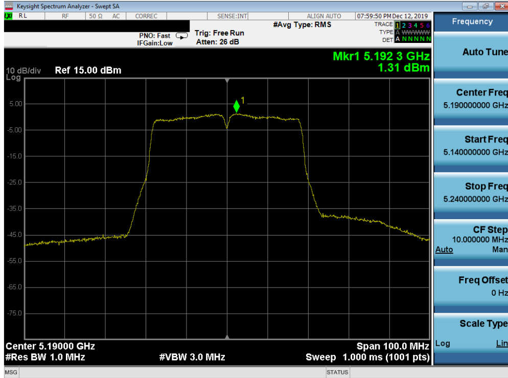
Plot 7-85. Power Spectral Density Plot SISO ANT1 (40MHz BW 802.11n (UNII Band 1) – Ch. 38)
