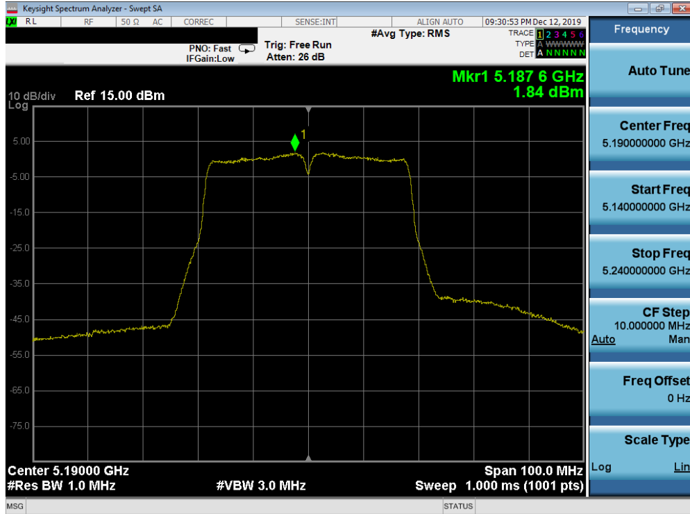
Plot 7-124. Power Spectral Density Plot SISO ANT2 (40MHz BW 802.11n (UNII Band 1) – Ch. 38)
