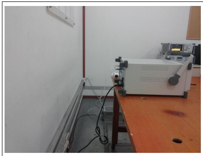
**- Photo of AC Power line emission Test - Bluetooth Low Energy, WLAN**
