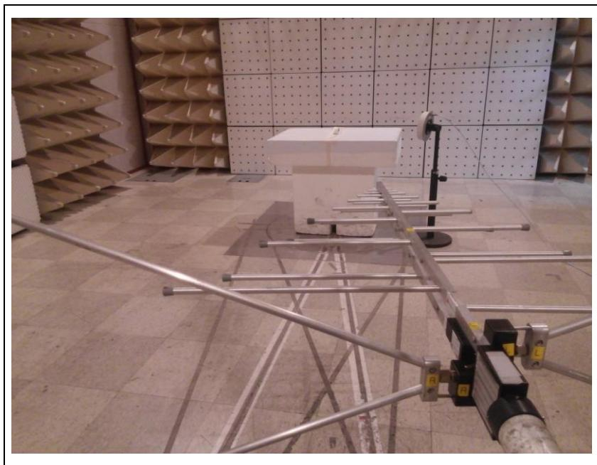
**- Photo of Radiated Spurious Emission Test (Above 1 GHz) - Bluetooth**
