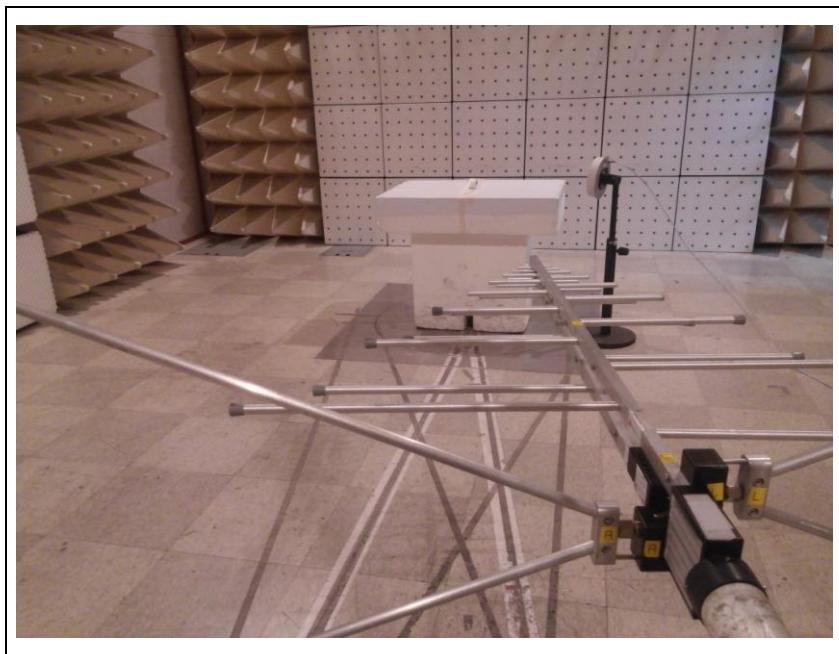
**- Photo of Radiated Spurious Emission Test (Above 1 GHz) - Bluetooth**
