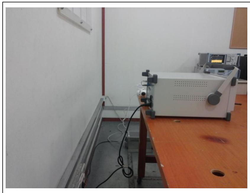
**- Photo of AC Power line emission Test - Bluetooth Low Energy, WLAN**
