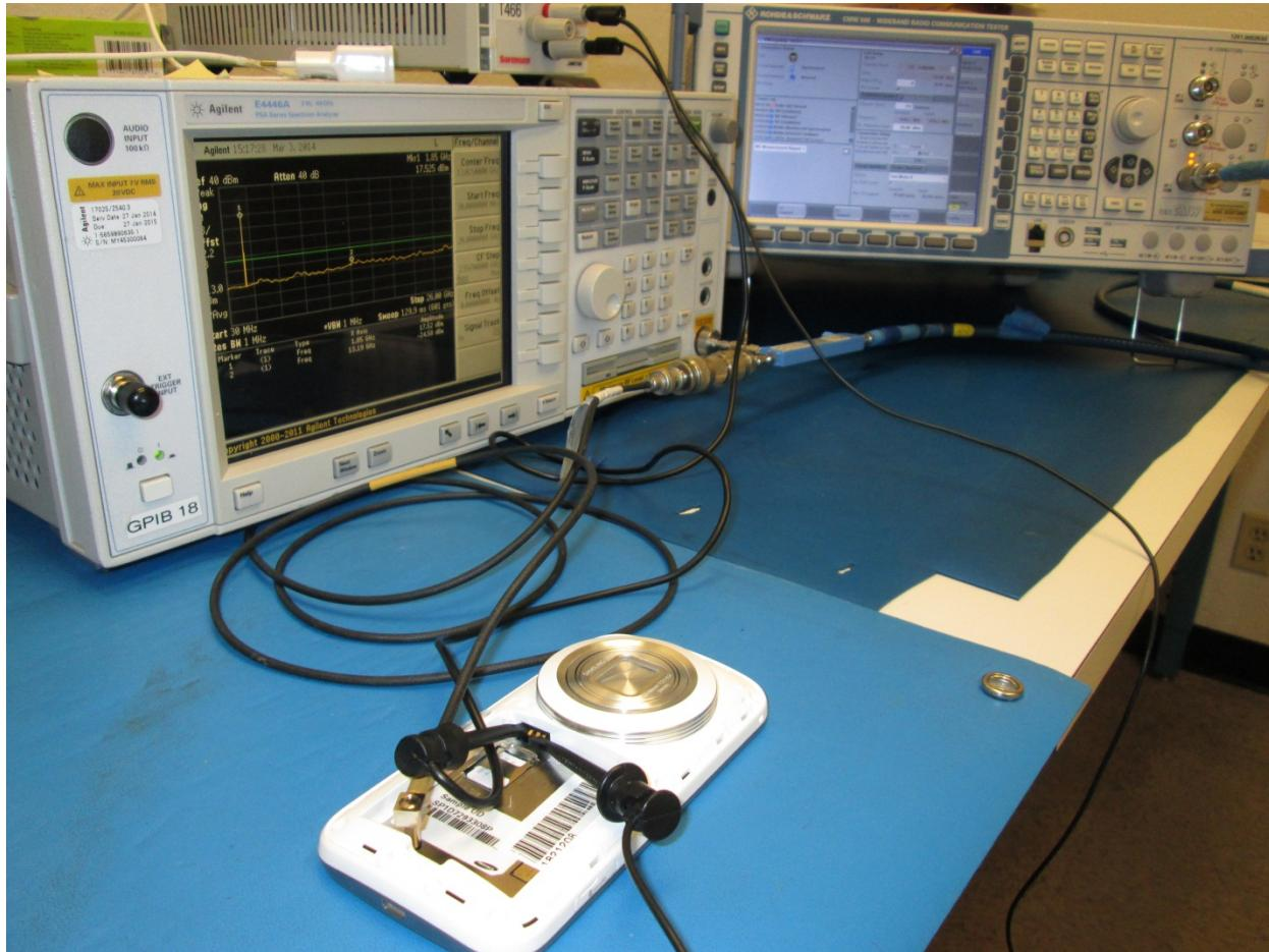
**RADIATED RF MEASUREMENT SETUP FOR PORTABLE CONFIGURATION**
