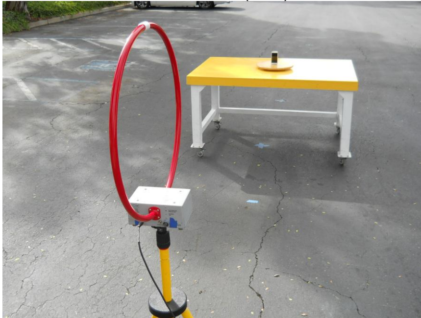
RADIATED EMISSIONS BELOW 30MHz (BACK)
