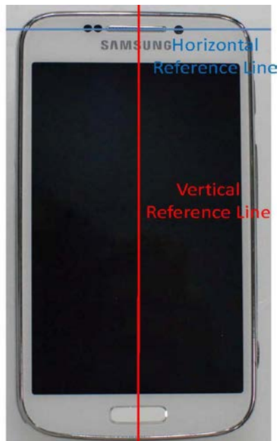
SAR Test Setup Photo 10 - Horizontal and Vertical Reference Lines
