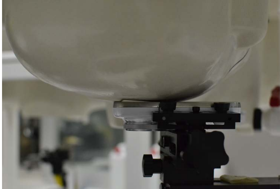
SAR Test Setup Photo 1 - Right Cheek
