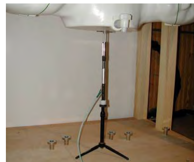
Figure 10-2 System Verification Setup Photo
