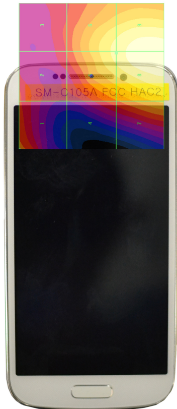
Figure 18-4 E-Field WD Scan overlay
