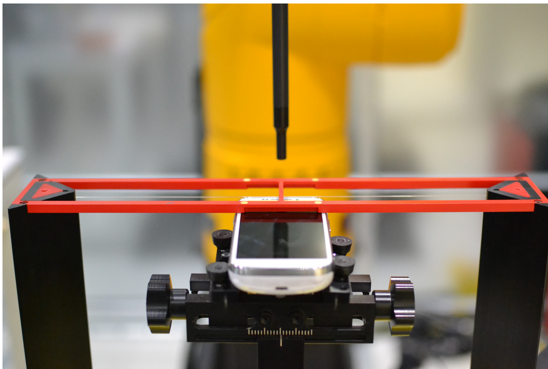
Figure 18-1 Ear Reference Point HAC Phantom Alignment
