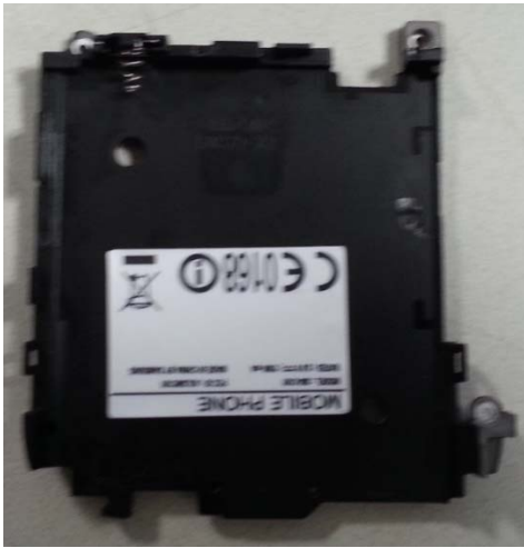
The FCC ID label is located in the battery compartment.
