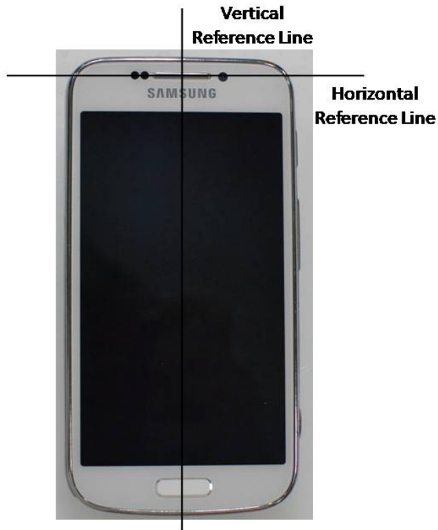
SAR Test Setup Photo 10: Vertical and Horizontal Reference Lines
