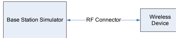
Figure 8-2 Power Measurement Setup
