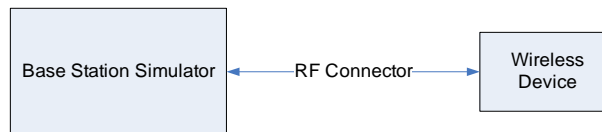
Figure 8-2 Power Measurement Setup
