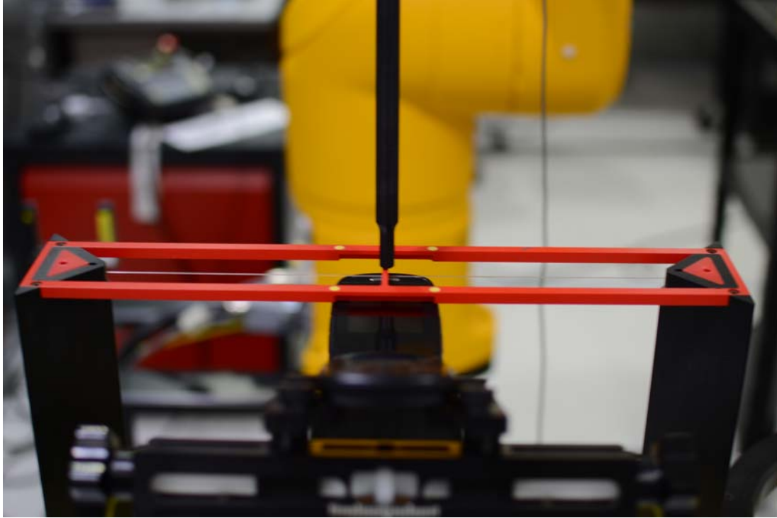
Figure 18-1 Ear Reference Point HAC Phantom Alignment
