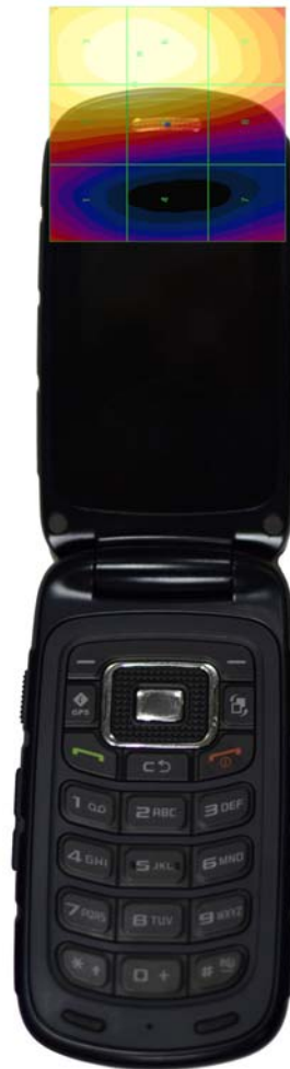
Figure 18-4 E-Field WD Scan overlay
