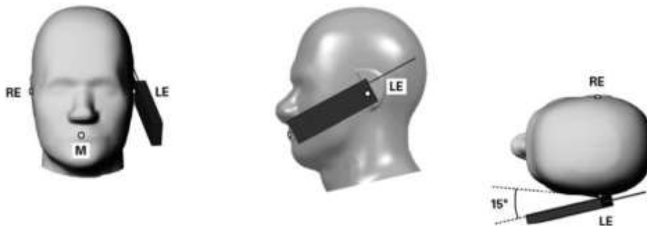
Figure 6.5. Tilt 15° position of the wireless device
