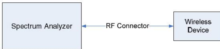
Figure 7-1. Test Instrument & Measurement Setup
