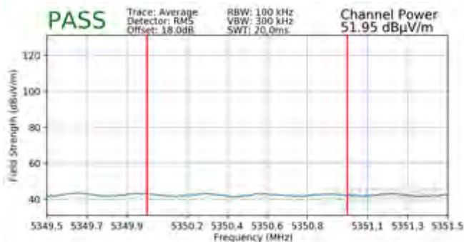
Plot 7-236. Radiated Upper Band Edge Plot MIMO (Average – UNII Band 2A)
