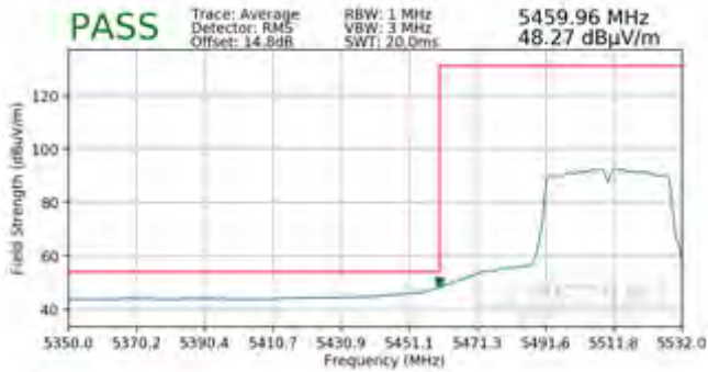
Plot 7-204. Radiated Lower Band Edge Plot SISO ANT2 (Average – UNII Band 2C)
