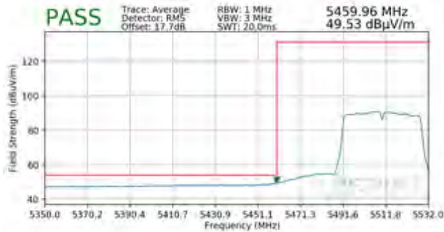
Plot 7-183. Radiated Lower Band Edge Plot SISO ANT1 (Average – UNII Band 2C)
