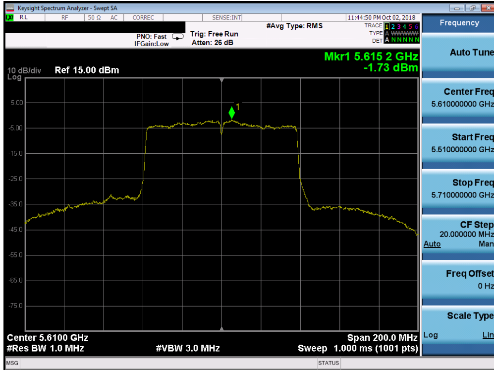
Plot 7-107. Power Spectral Density Plot SISO ANT1 (80MHz BW 802.11ac (UNII Band 2C) – Ch. 122)
