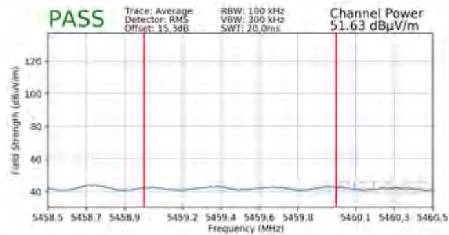
Plot 7-211. Radiated Lower Band Edge Plot SISO ANT2 (Average – UNII Band 2C)
