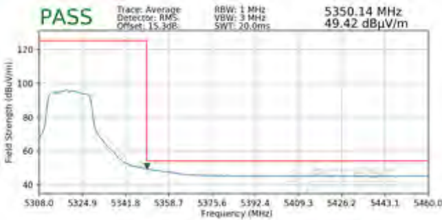
Plot 7-174. Radiated Upper Band Edge Plot SISO ANT1 (Average – UNII Band 2A)
