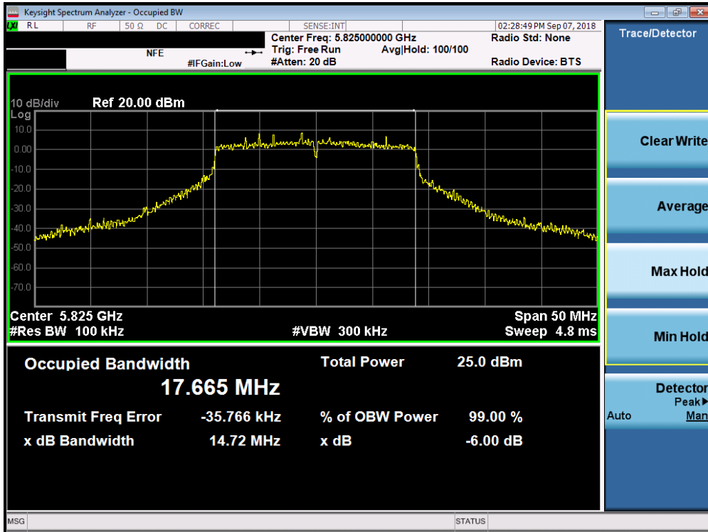
Plot 7-66. 6dB Bandwidth Plot SISO ANT1 (20MHz BW 802.11n (UNII Band 3) – Ch. 165)
