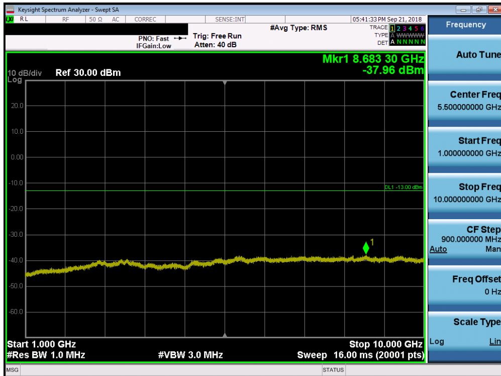
Plot 7-21. Conducted Spurious Plot (LTE Band 26, 1.4MHz QPSK – RB Size 1, RB Offset 0 – High Channel)
