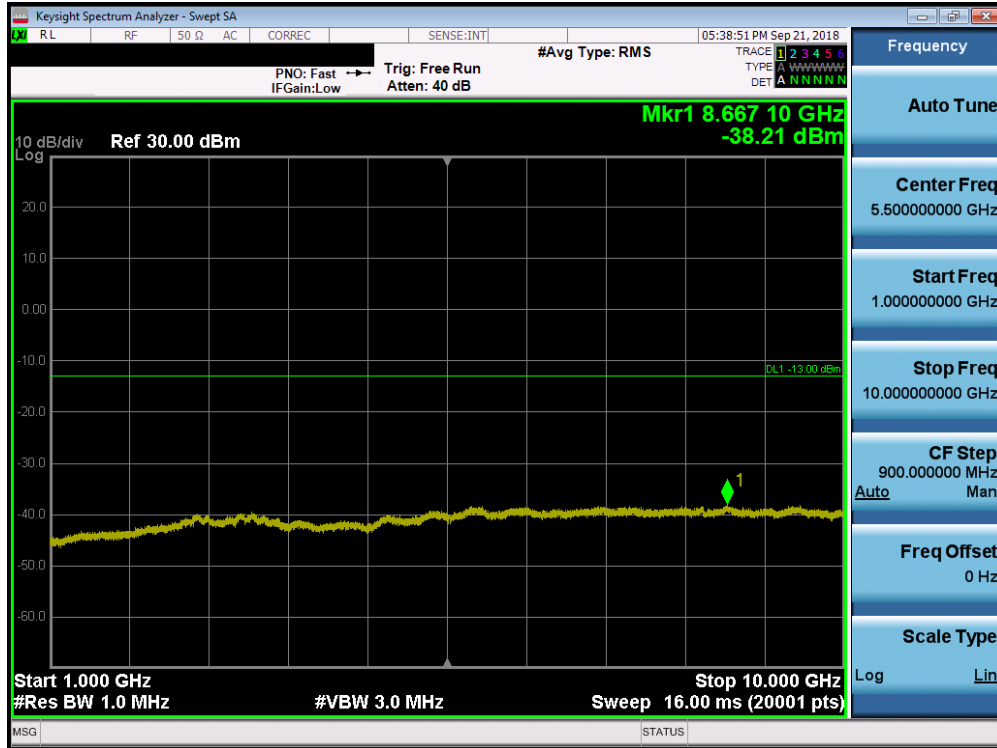
Plot 7-18. Conducted Spurious Plot (LTE Band 26, 1.4MHz QPSK – RB Size 1, RB Offset 0 – Low Channel)
