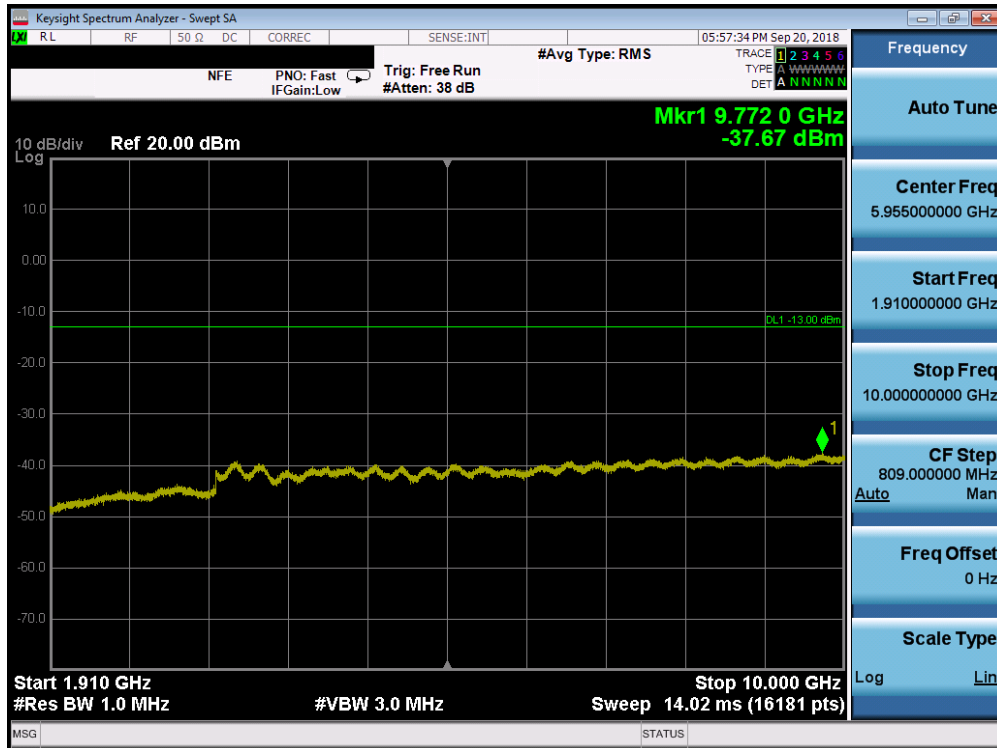
Plot 7-113. Conducted Spurious Plot (Band 2 - 10.0MHz QPSK - RB Size 1, RB Offset 0 - Low Channel)
