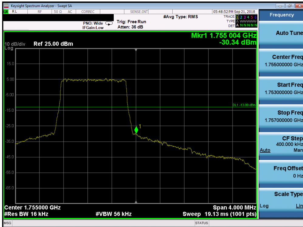
Plot 7-160. Upper Band Edge Plot (Band 4 - 1.4MHz QPSK - Full RB Configuration)
