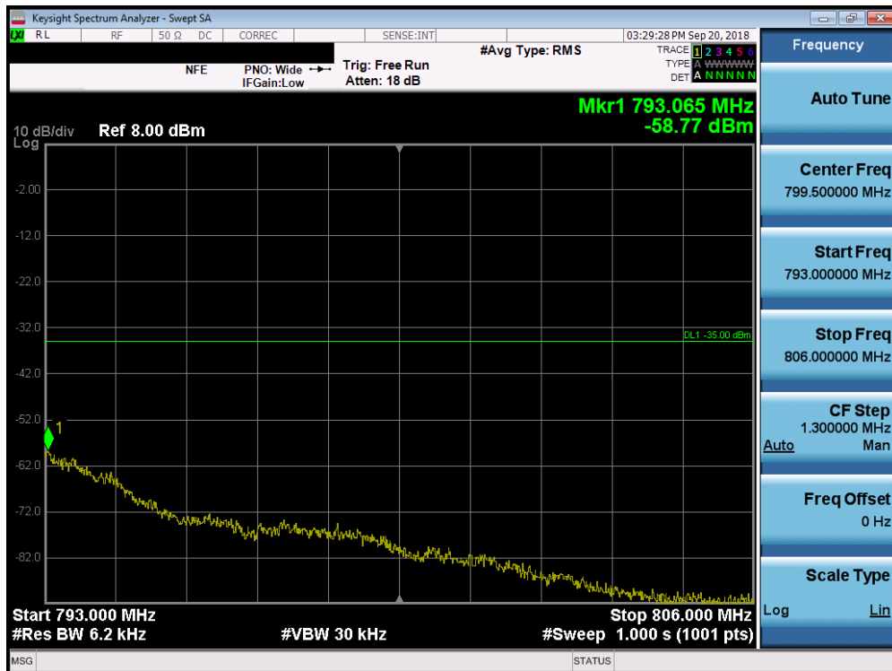
Plot 7-143. Upper Emission Mask Plot (Band 13 - 5.0MHz QPSK - Full RB Configuration)
