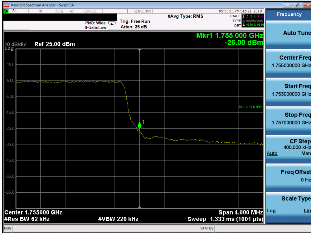
Plot 7-172. Upper Band Edge Plot (Band 4 - 5.0MHz QPSK - Full RB Configuration)
