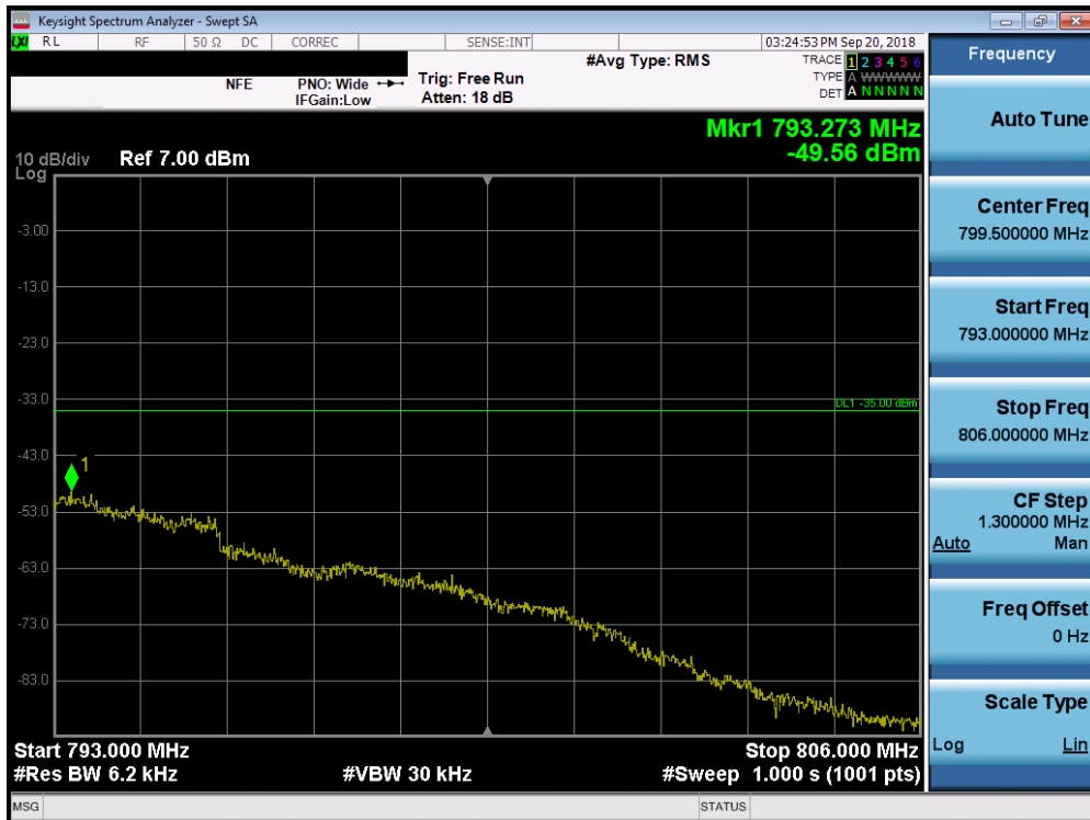
Plot 7-147. Upper Emission Mask Plot (Band 13 - 10.0MHz QPSK - Full RB Configuration)
