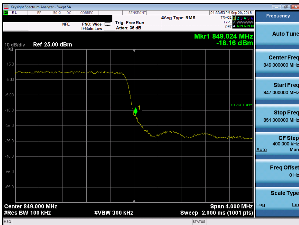
Plot 7-151. Upper Band Edge Plot (Band 26/5 - 3.0MHz QPSK - Full RB Configuration)
