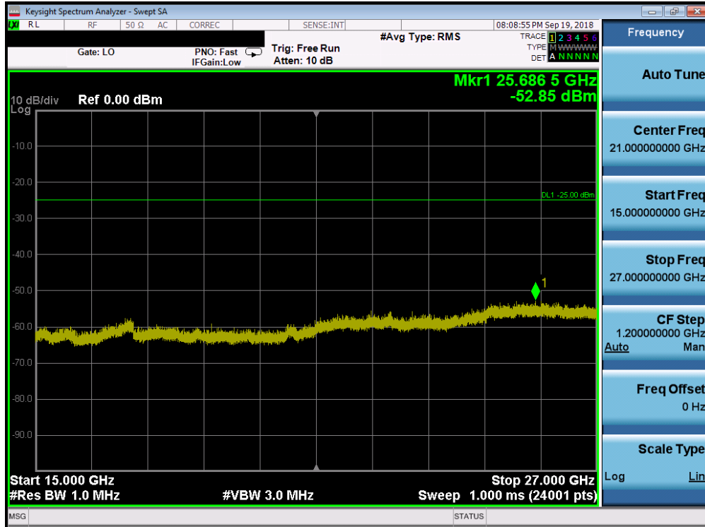
Plot 7-129. Conducted Spurious Plot (Band 41 - 10.0MHz QPSK - RB Size 1, RB Offset 0 - High Channel)
