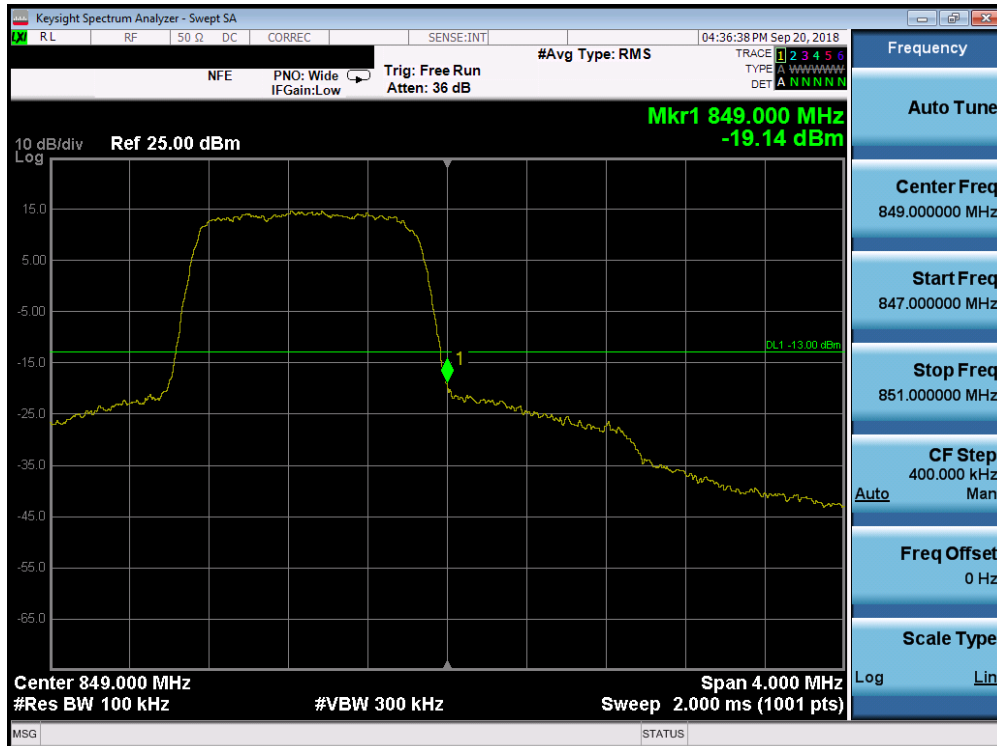
Plot 7-149. Upper Band Edge Plot (Band 26/5 - 1.4MHz QPSK - Full RB Configuration)
