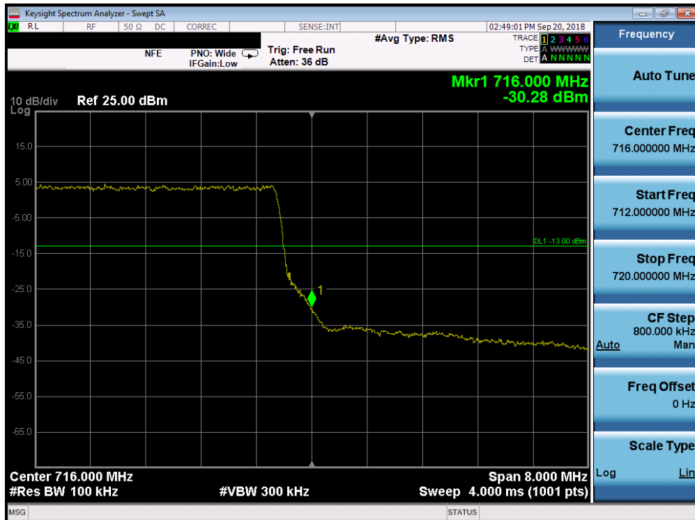
Plot 7-139. Upper Band Edge Plot (Band 12/17 - 10.0MHz QPSK - Full RB Configuration)
