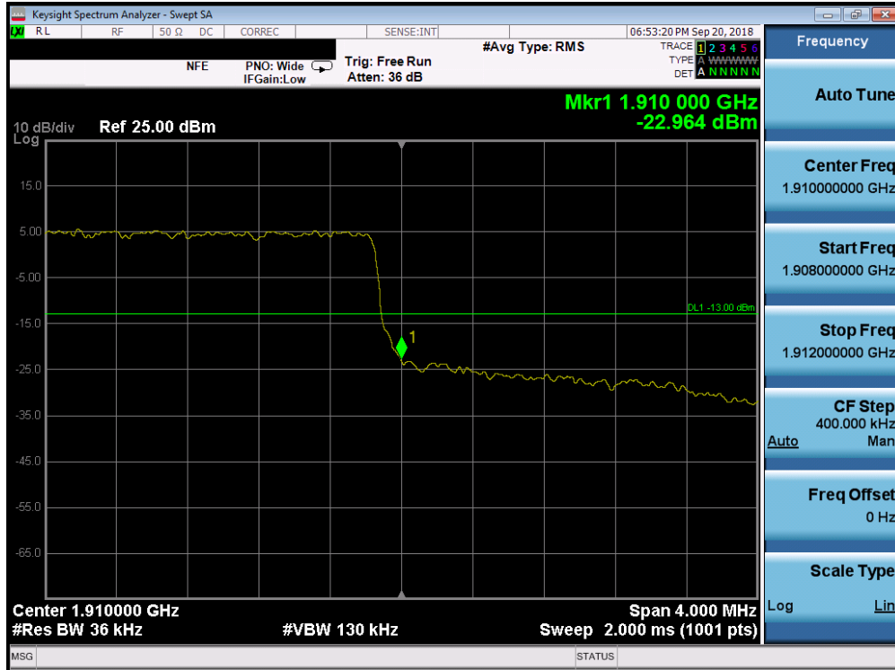
Plot 7-200. Upper Band Edge Plot (Band 2 - 3.0MHz QPSK - Full RB Configuration)
