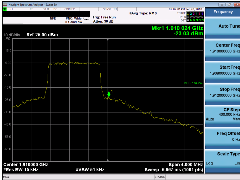
Plot 7-196. Upper Band Edge Plot (Band 2 - 1.4MHz QPSK - Full RB Configuration)
