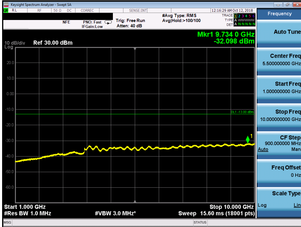
Plot 7-90. Conducted Spurious Plot (Band 12/17 - 10.0MHz QPSK - RB Size 1, RB Offset 0 - High Channel)
