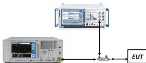
Figure 7-3. Test Instrument & Measurement Setup
