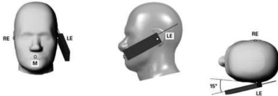
Figure 8.5. Tilt 15° position of the wireless device
